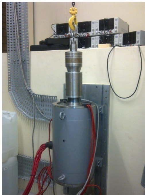
Figure 5-18: Assembling the IM rotor into the stator
