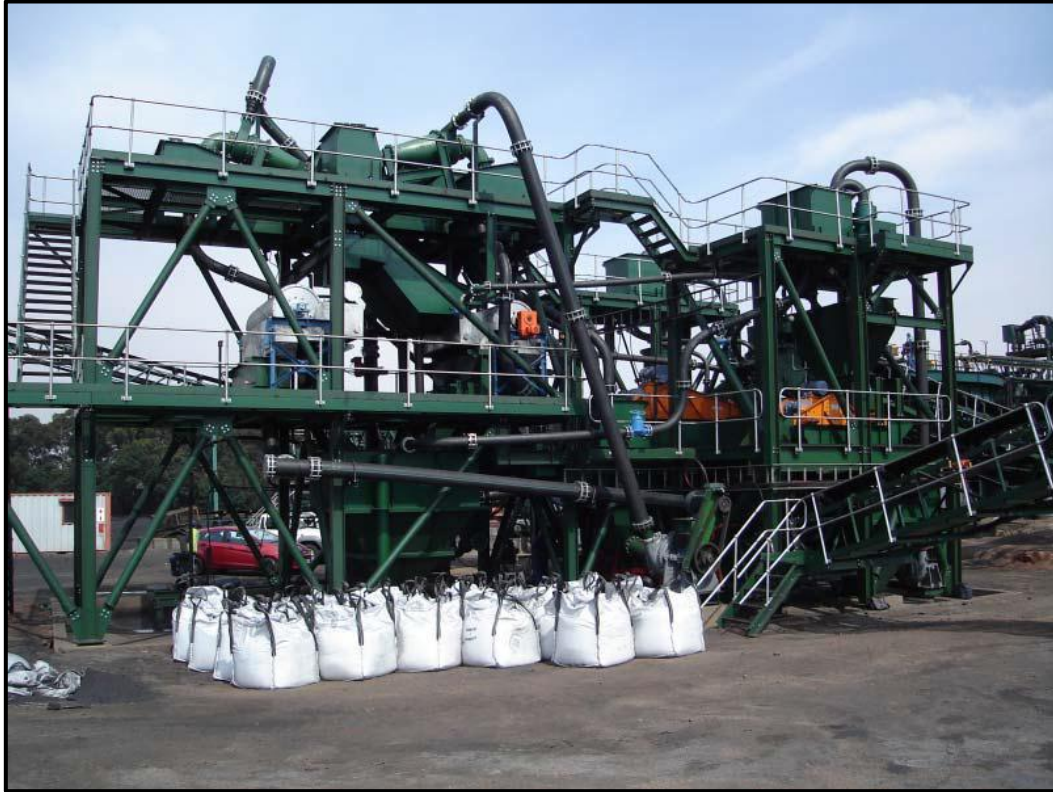
Figure 2-1: Muhanga's fine coal dense-medium cyclone beneficiation plant (De Korte, 2014)
