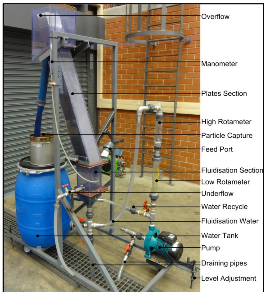
Figure 3-11: The completed RC105 unit and descriptions
