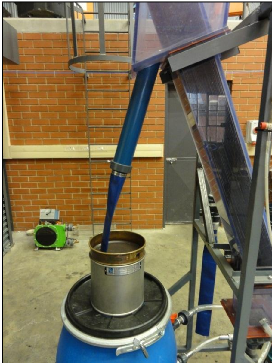
Figure 3-13: Batch mode overflow configuration
