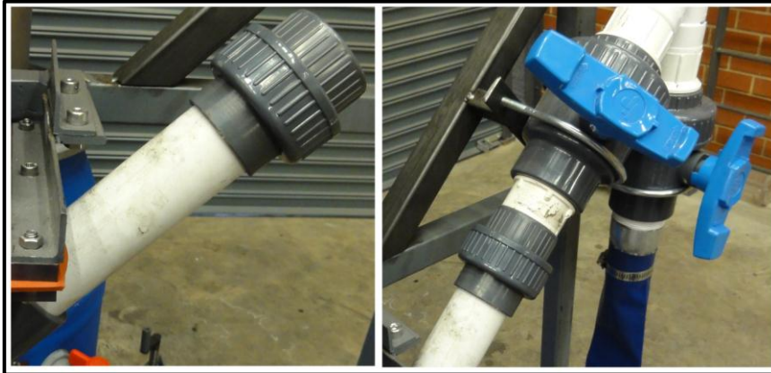
Figure 3-4: Illustrating the plug and the pipe configuration that is fastened to the female PVC union fitting
