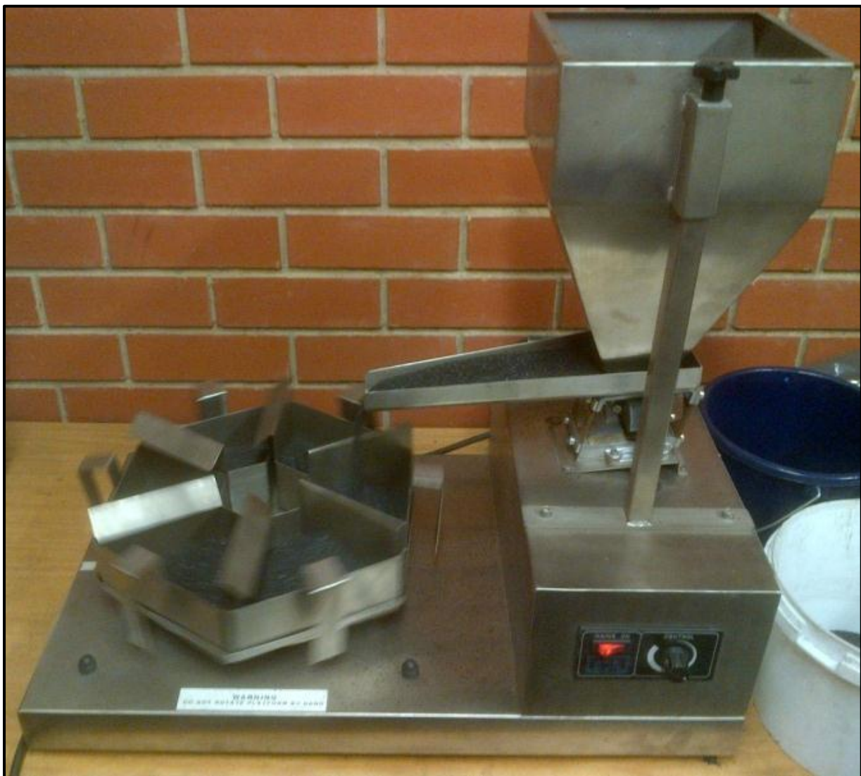
Figure 3-14: Photo of the spinning riffler sample divider
