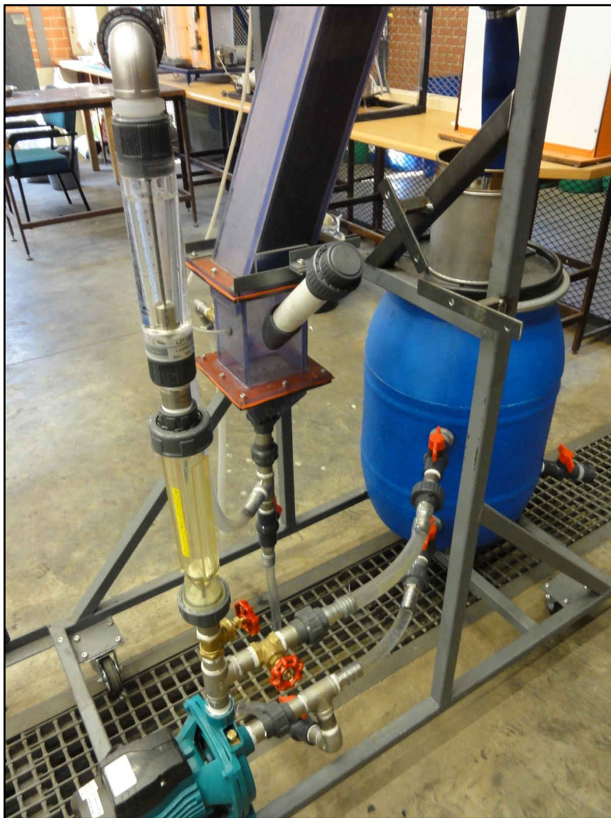
Figure C-2: Photo – Rotameters and piping
