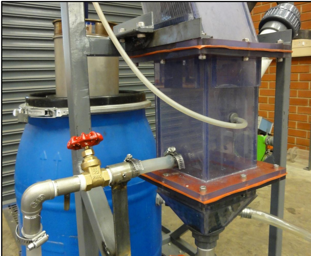
Figure C-5: Photo – Fluidisation section, discard and manometer
