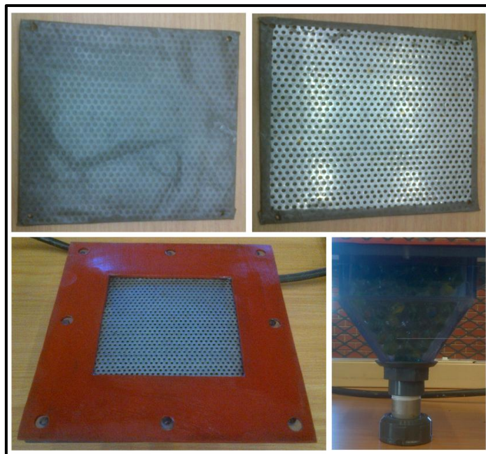
Figure 3-8: Photos of the 75 \mu\text{m} wire mesh, perforated plate and flow distribution part filled with marbles
