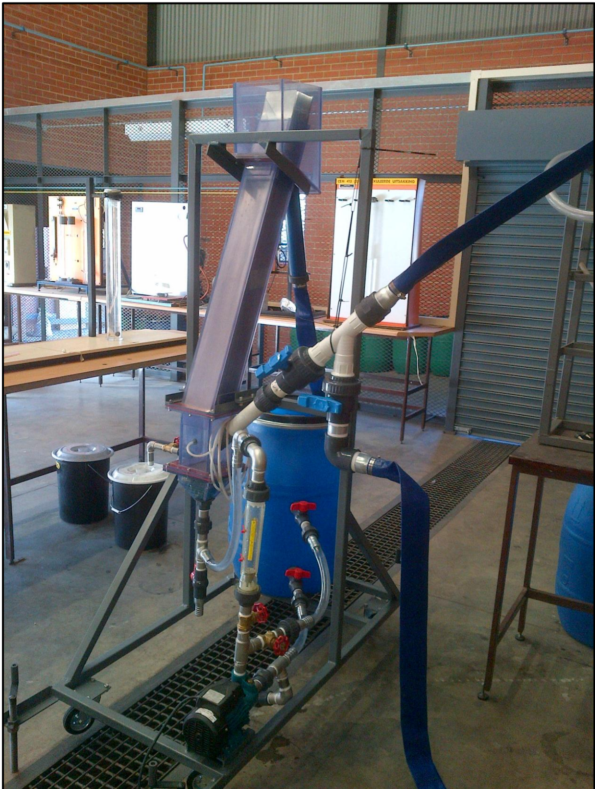
Figure C-9: Photo – Initial stage of valve and pipe configuration of semi-batch feeding system
