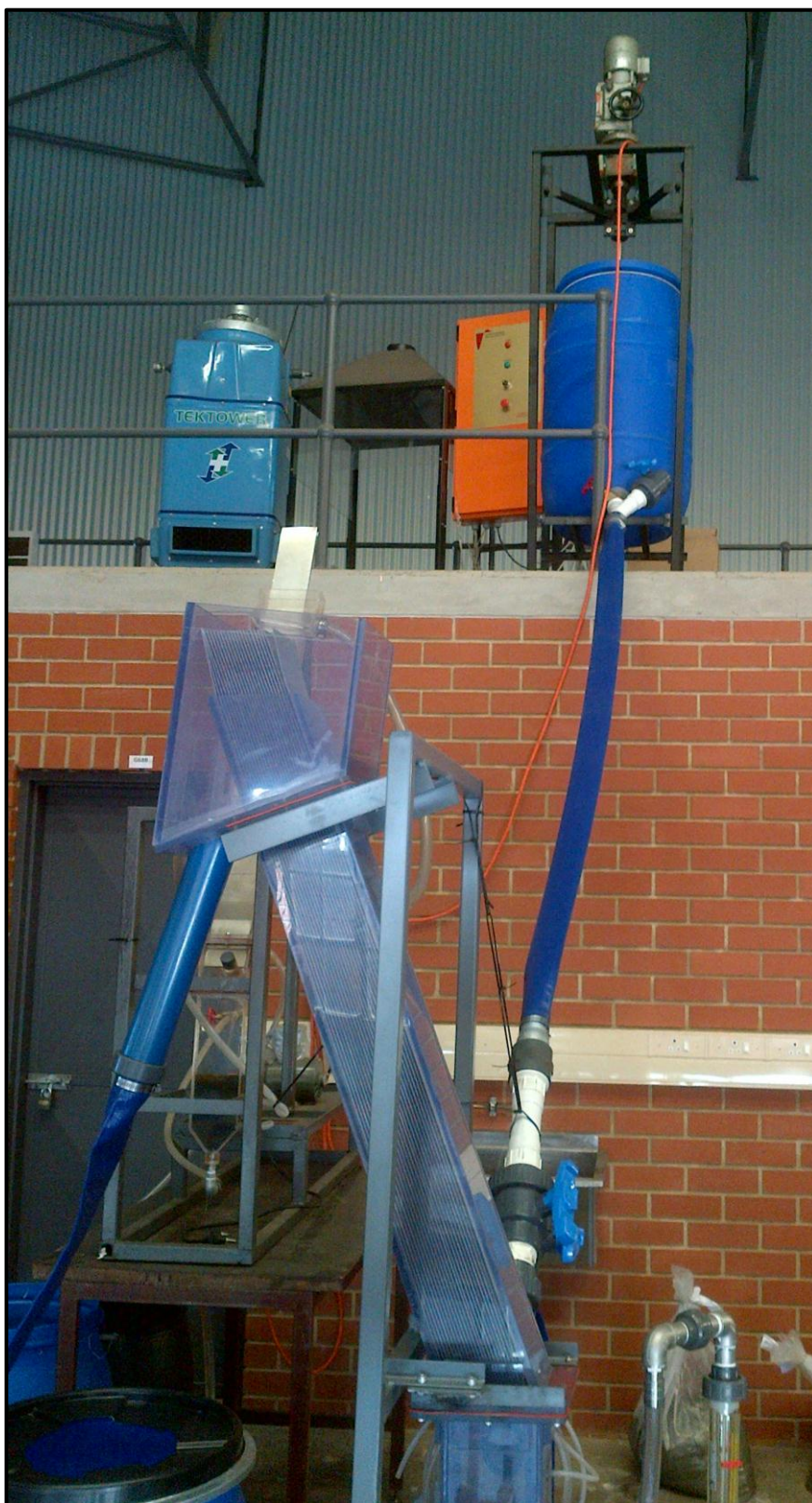
Figure C-8: Photo – Gravity feeding of unit during semi-batch mode
