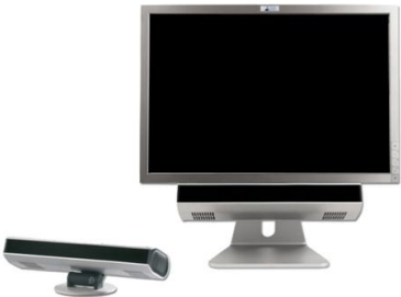
Figure 13: SMI's iViewX™ RED500 eye-tracking system
