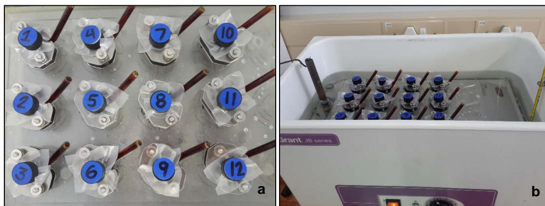
Figure 5.4: Assembled vertical Franz diffusion cells: (a) placed on a magnetic stirrer plate and b) in a temperature controlled water bath system.
