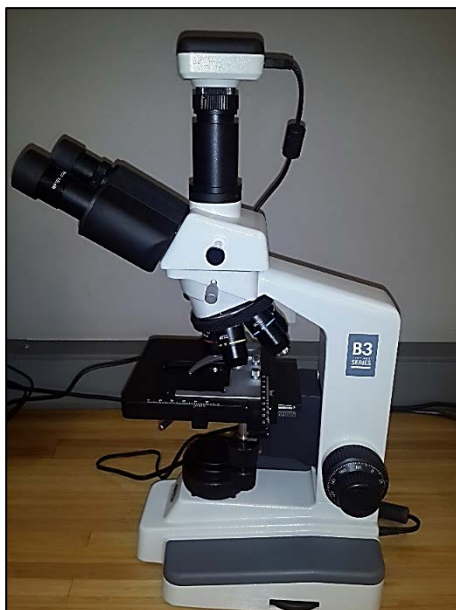
Figure 4.6: Motic microscope, equipped with a Moticam 3 camera that uses Motic Images Plus software.
