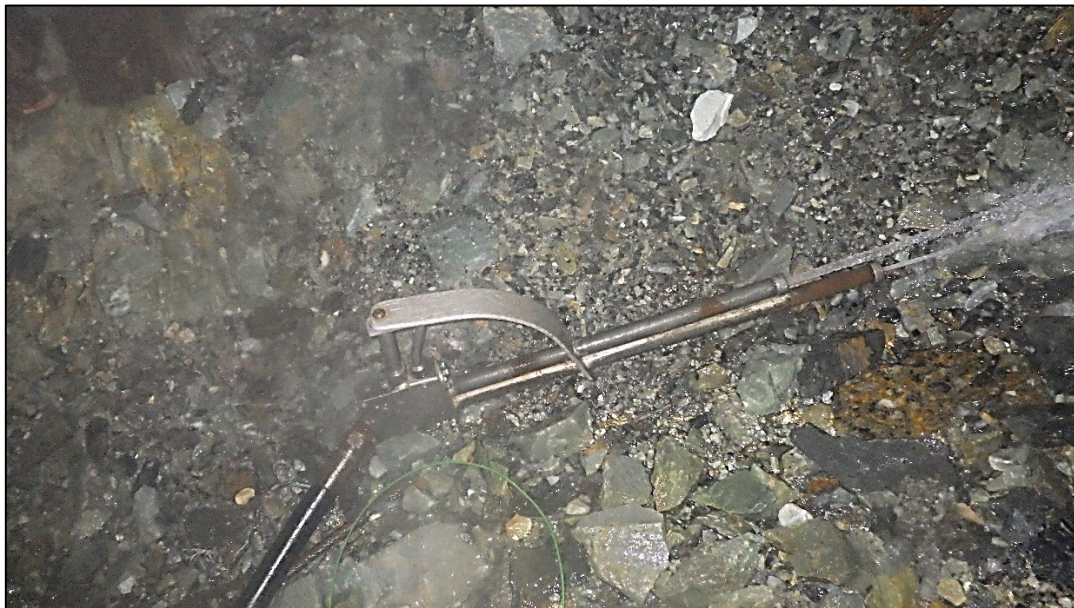
Figure 3-15: Open water jet left unattended
