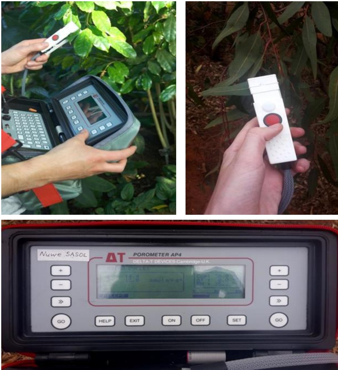
Figure 45: Measuring stomatal conductance through Delta-T AP4 Leaf Porometer
