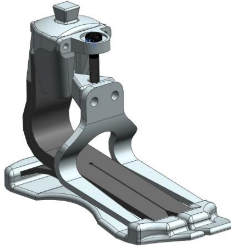
Figure 32: Vertically adjusting blades: fork design concept.
