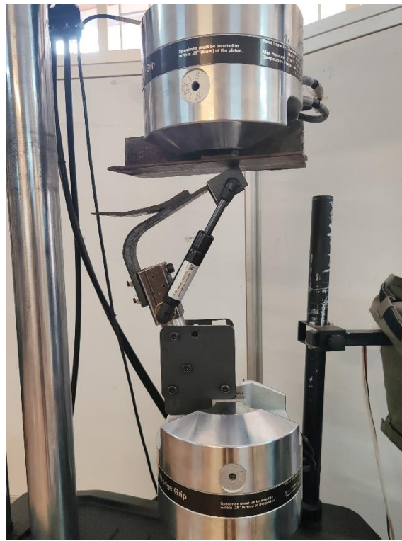
Figure 67: Prosthetic foot during testing with two 500 N gas springs attached
