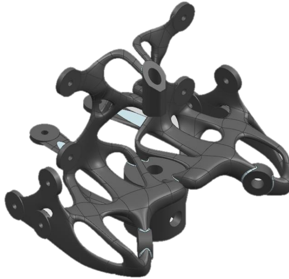
Figure 5-35: The final geometry of the current biomimetic bottom bracket
