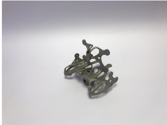
Figure 5-33: Second build result for the current biomimetic bracket
