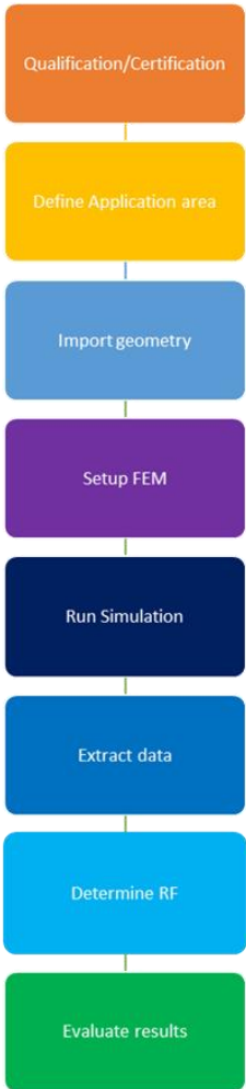
Figure 5-38: Qualification and certification process flow
