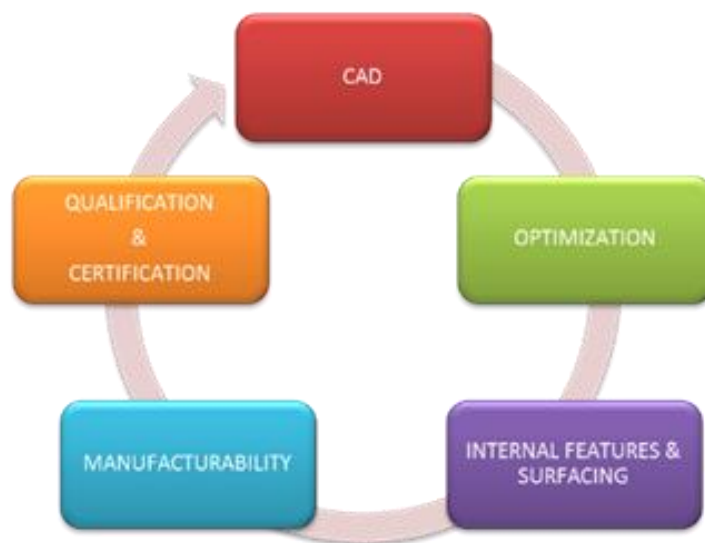
Figure 3-1: The design cycle for additively manufactured aerospace components
