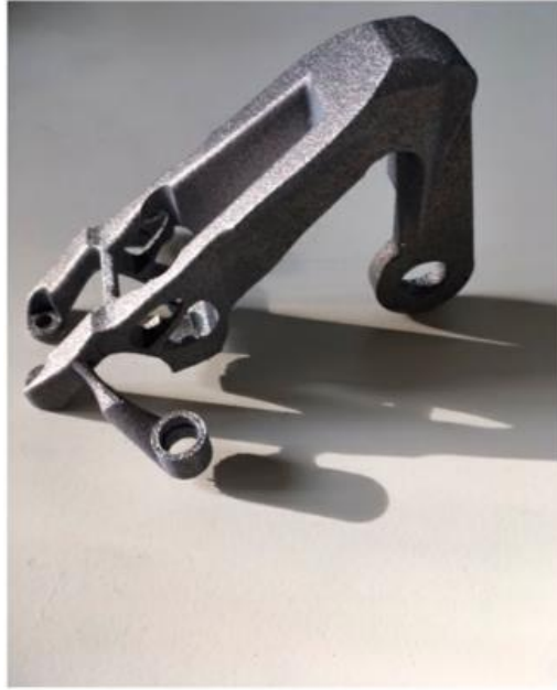
Figure 2-2: Ti64 component printed with the LBPf process
