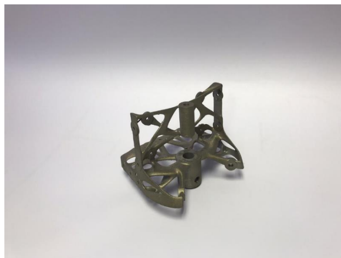
Figure 5-32: Second build result for the volumetric biomimetic bracket
