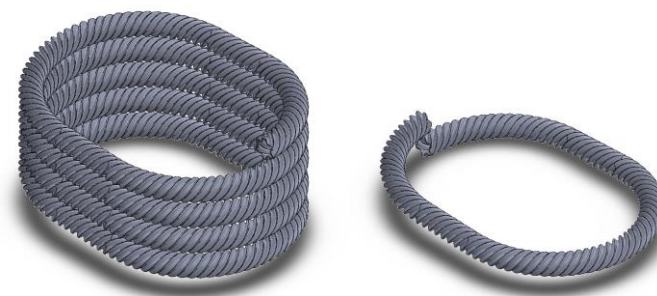
Figure 3-28: Entire HCFT-HX with 4.5 coil revolutions (left) and a single revolution (right)
