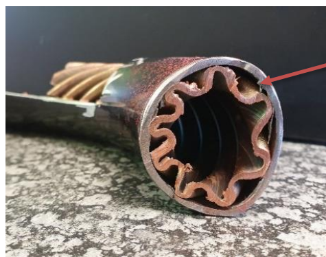
Figure 1-3: Cross-section of a copper HCFT-HX manufactured using traditional technology.
