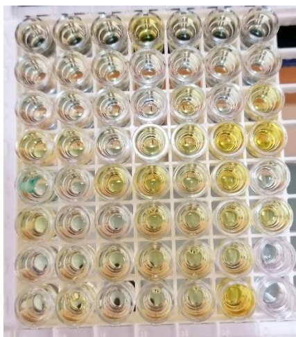
Figure 3-4: Image of a completed glyphosate ELISA test prior to spectrophotometry at 450 nm
