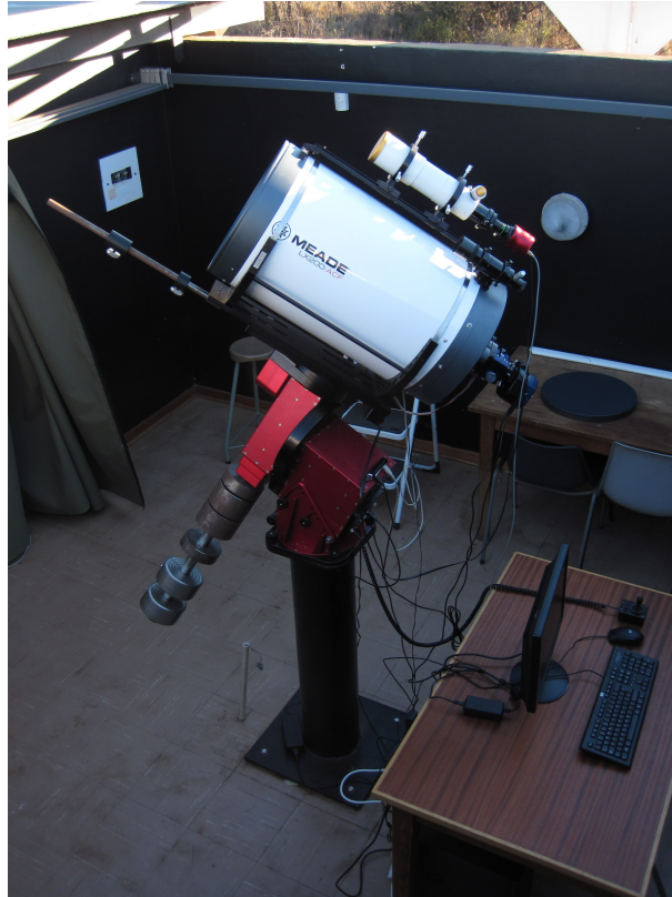
FIGURE 3.1: The new 16 inch telescope setup on the small observatory, Nooitgedacht, of the North-West University, where the more recently installed autoguiding system can also be seen.
