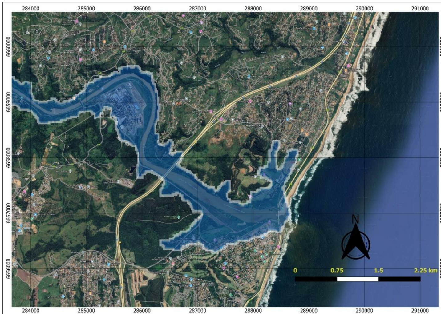
Figure 4–9: Flood extent map generated from HEC-RAS hydraulic modelling, showing the spatial distribution of inundated areas along uMkomazi River during the simulated flood event.
