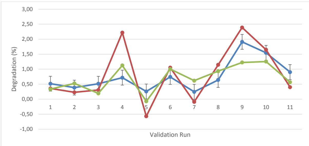
Figure 5.8 Comparison of the predicted and observed values for the validation of the abrasion resistance models ● observed ● linear with interactions ● second order model
