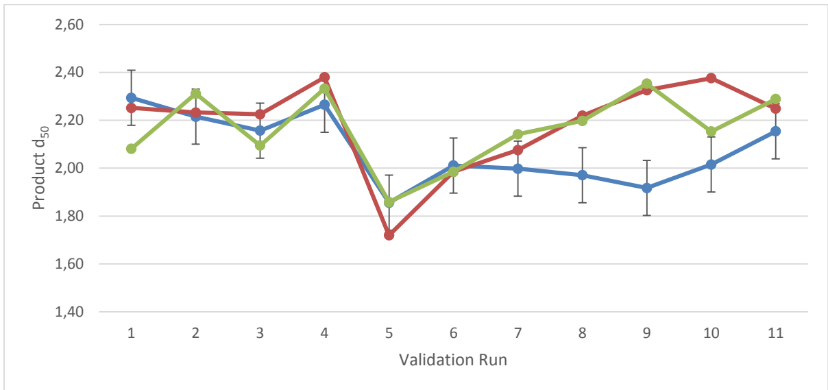
Figure 5.11 Comparison of the predicted and observed values for the validation of the product size models ● observed ● linear with interactions ● second order model
