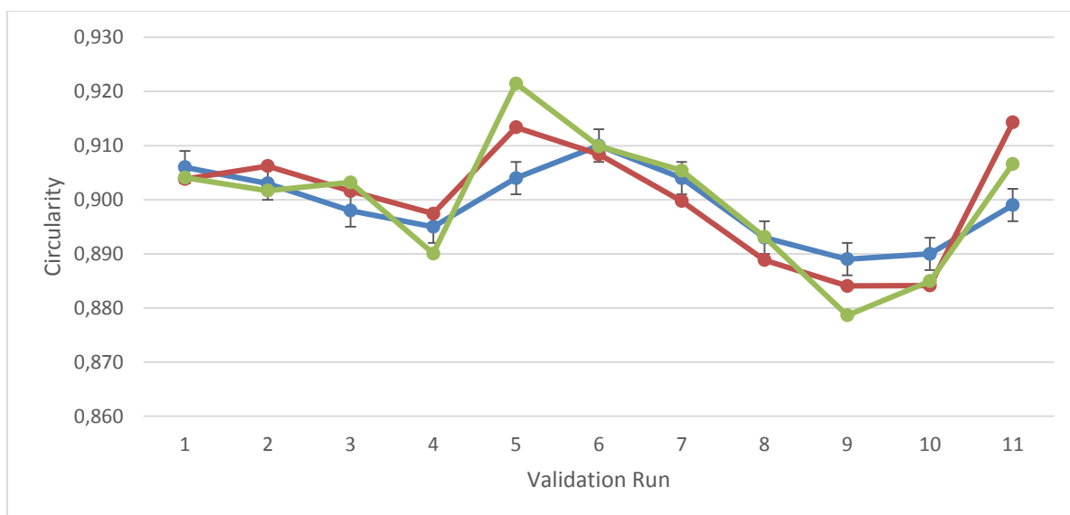
Figure 5.14 Comparison of the predicted and observed values for the validation of the product shape models ● observed ● linear with interactions ● second order model
