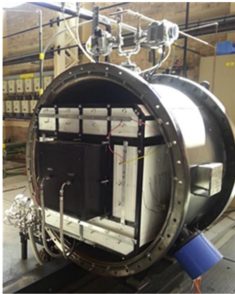
Figure 2.8: A photo of the NWTCTF vessel and internals (left) and exploded view of the test section components (right) from (De Beer, et al., 2018).
