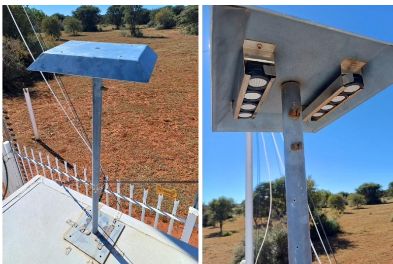
Figure 3.2 The housing unit used for deployment of passive samplers at Welgegund with the aluminium rails in which the passive samplers were placed shown on the right.
