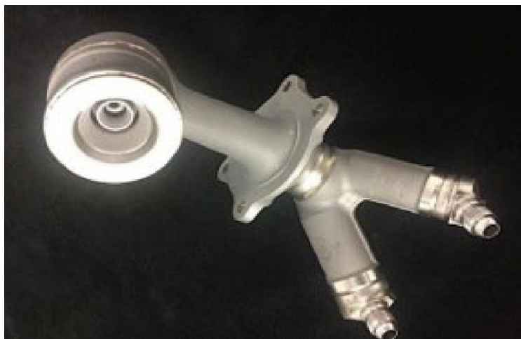
Figure 2.4-2: GE's fuel nozzle, which has been additively manufactured [12]
