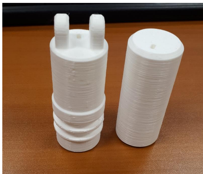
Figure 2.2-5: Support material removed from parts
