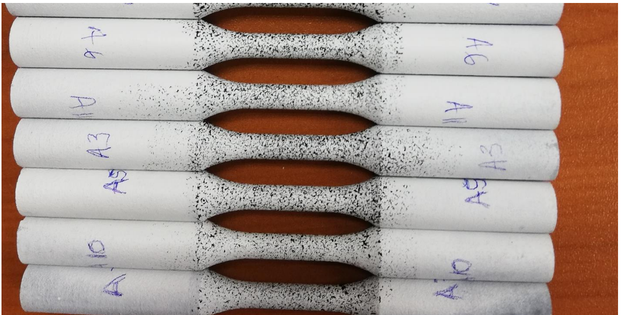
Figure 4.3-2: Test samples once the speckle pattern has been applied
