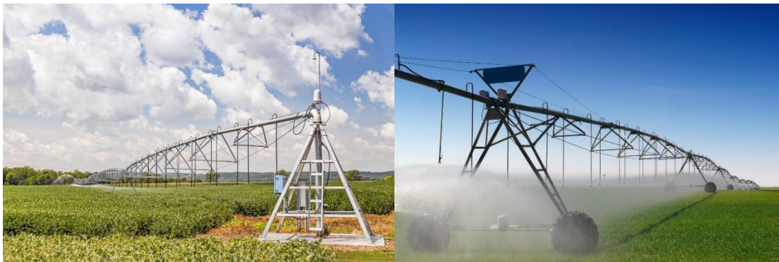
Figure 21: a) Centre pivot with a control panel, and b) Pivot irrigation structure irrigating [88]
