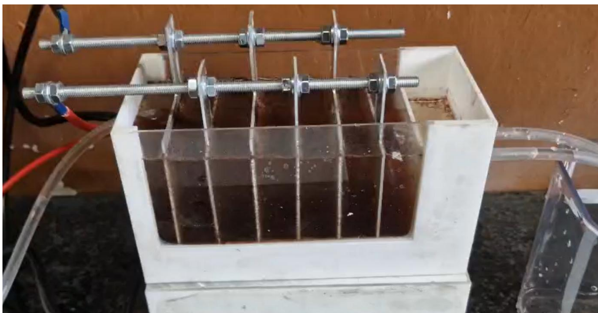
Figure 39: EC reactor - de-energised
