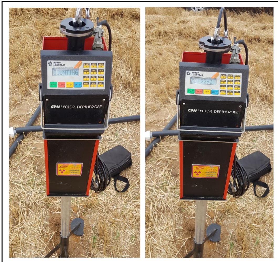
Figure 7: To the left, the control unit showing that it is busy taking a measurement (count ratio). To the right, the measurement given by the control unit at a specific location.
