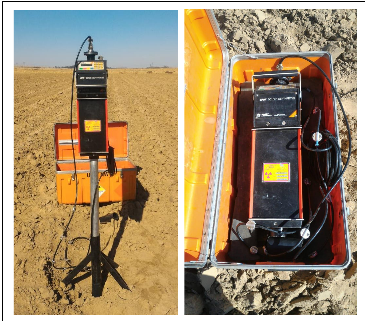
Figure 16: To the left, the Neutron probe is shown where it was placed on top of the tripod stand. To the right, the Neutron probe is placed in the protective carrycase.
