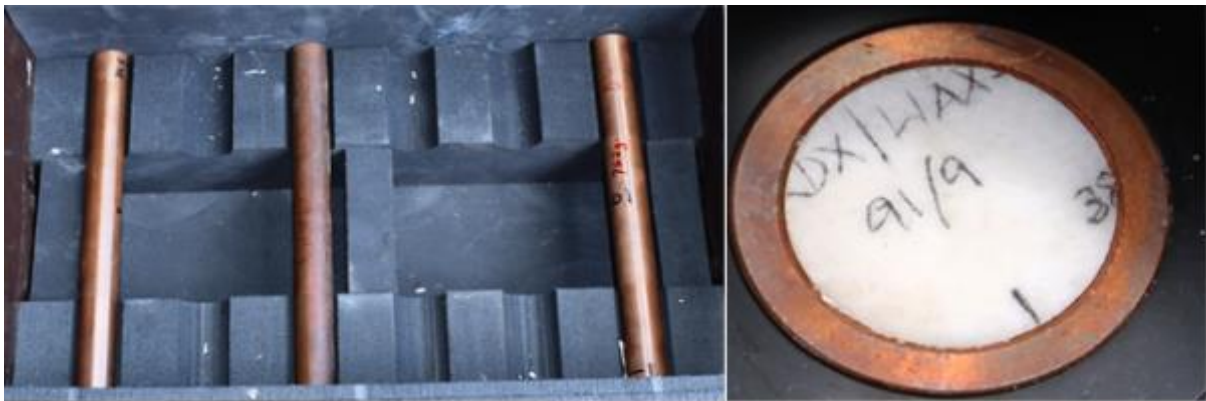
Figure 21: OFHC cylinder filled with explosive charges
