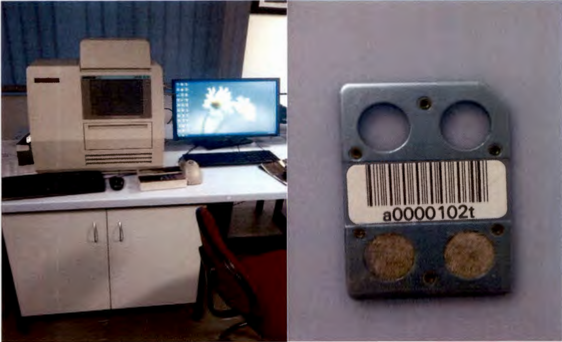
Figure 7: The 6600 Harshaw TLD reader (LHS) and the Thermo-Luminescence dosimeter (TLD 0011) (RHS) with positions iii) and iv) covered with the sample aliquots
