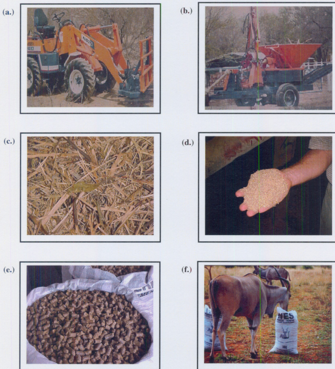
Figure 5.13 a-f: Wes Voere manufacturers of organic feed produced from wood of problem woody species in South Africa. (a.) Mechanical removal (cutting) of bushes; (b. - c.) Collection of all cut material (stems/ branches/ leaves) and shredding it to a finer texture and then; (d.) Mulching material by forcing it through a hammermill; (e.) and adding necessary nutrients and finally compressing it into pellets that can be (f.) fed to game.
