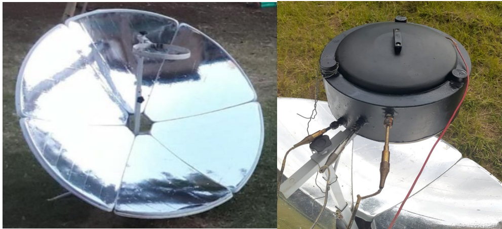
Figure 5.1: Photograph of the parabolic dish solar cooker with TES system implemented in the cooking pot. Left: parabolic solar collector, right: cooking pot with TES system
