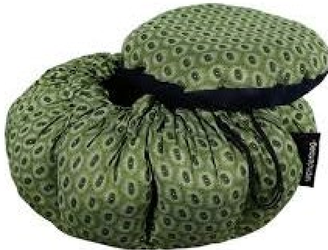
Figure 3.4: A photograph of the insulating wonderbag slow cooker used for heat retention cooking tests.
