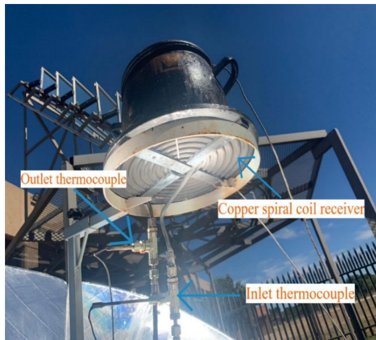
Figure 7.2: A photograph showing the main components of the receiver.
