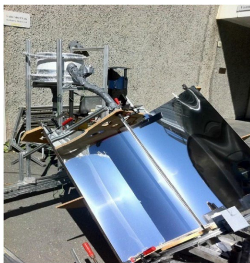
Figure 2.7: A photograph of a parabolic trough cooker integrated with LHTES. The figure was reproduced from Ref. [87], with the permission of Elsevier Publishing.
