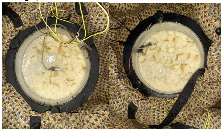
Figure 3.8: Rice and potatoes cooked with water using the wonderbags combined with (a) the oil storage cooking pot and (b) the erythritol storage cooking pot on 28 February 2020.
