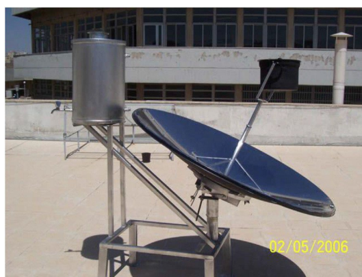
Figure 2.5: A photograph of the experimental setup of a portable solar cooker and water heater. The figure was reproduced from Ref. [73], with the permission of Elsevier Publishing.
