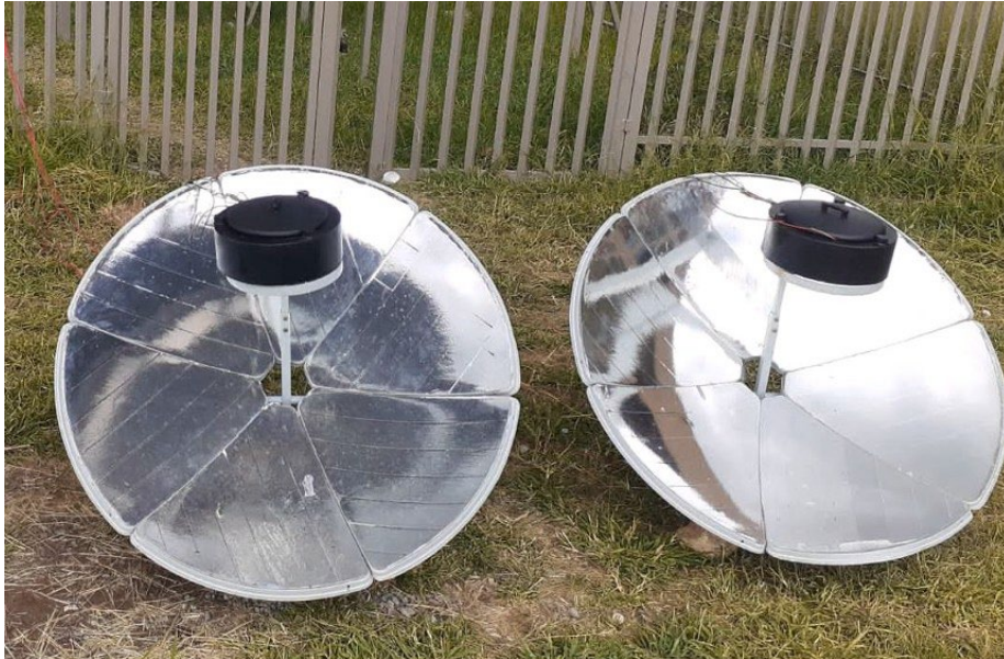
Figure 3.5: Experimental testing of the two storage cooking pots with two parabolic dish solar cookers.
