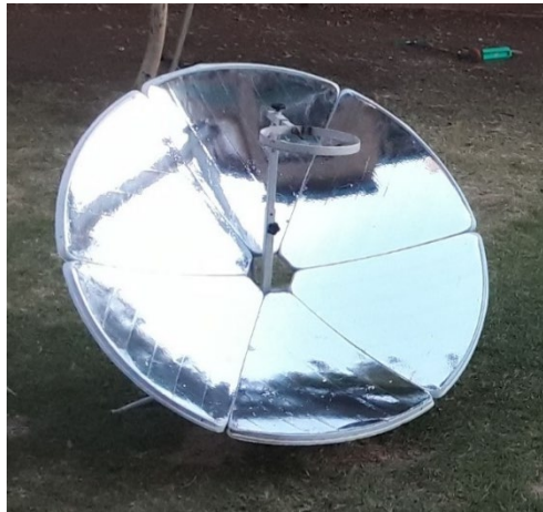
Figure 3.1: A photograph of the parabolic dish solar cooker used in the cooking tests.
