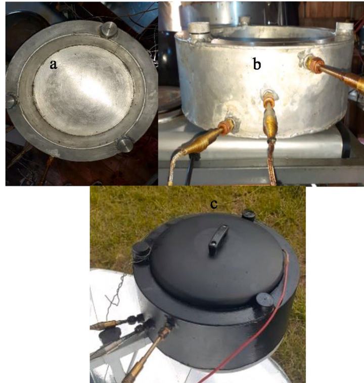
Figure 3.2: Photographs of the storage cooking pot; (a) plan view, (b) side view and (c) the storage cooker painted black in a solar cooking experiment.
