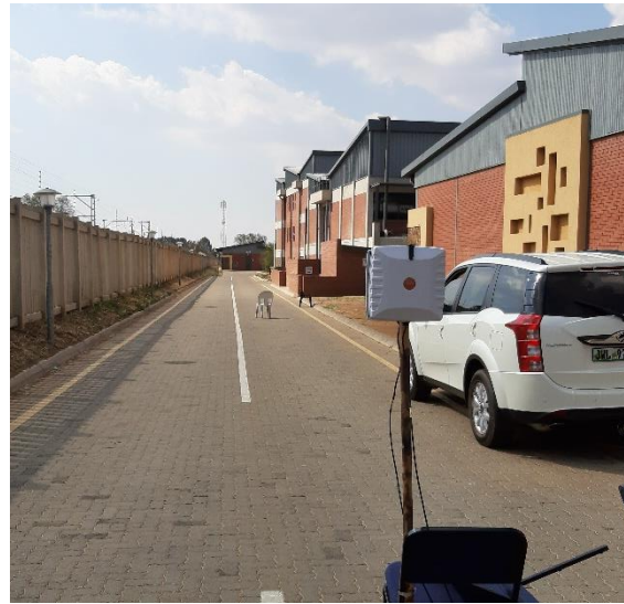
Figure 5-9: Experimental setup to test the effect of reflections on the motion estimation techniques
