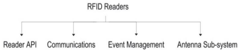
Figure 2-4: Functions of a RFID reader, reproduced from [33]
