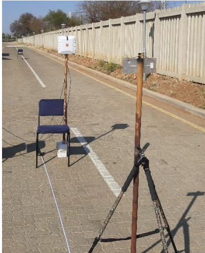
Figure 5-5: Characterizing the RFID tag at a fixed distance (back view)
