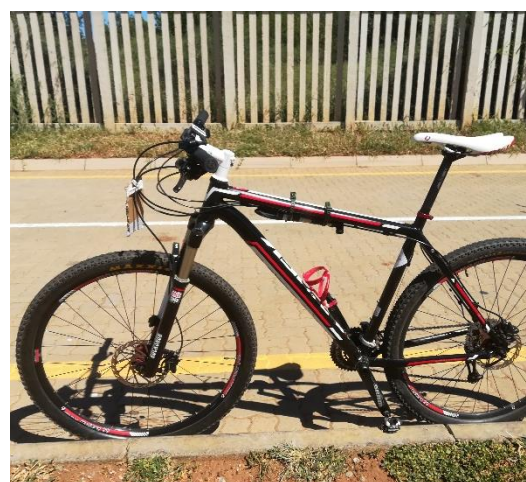
Figure 5-4: Tag placement on bicycle for practical measurements, where the tag is oriented with the ideal angle in reference to the antennas
