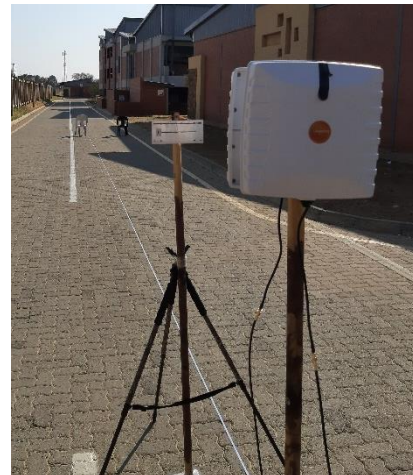
Figure 5-6: Characterizing the RFID tag at a fixed distance (Front view)
