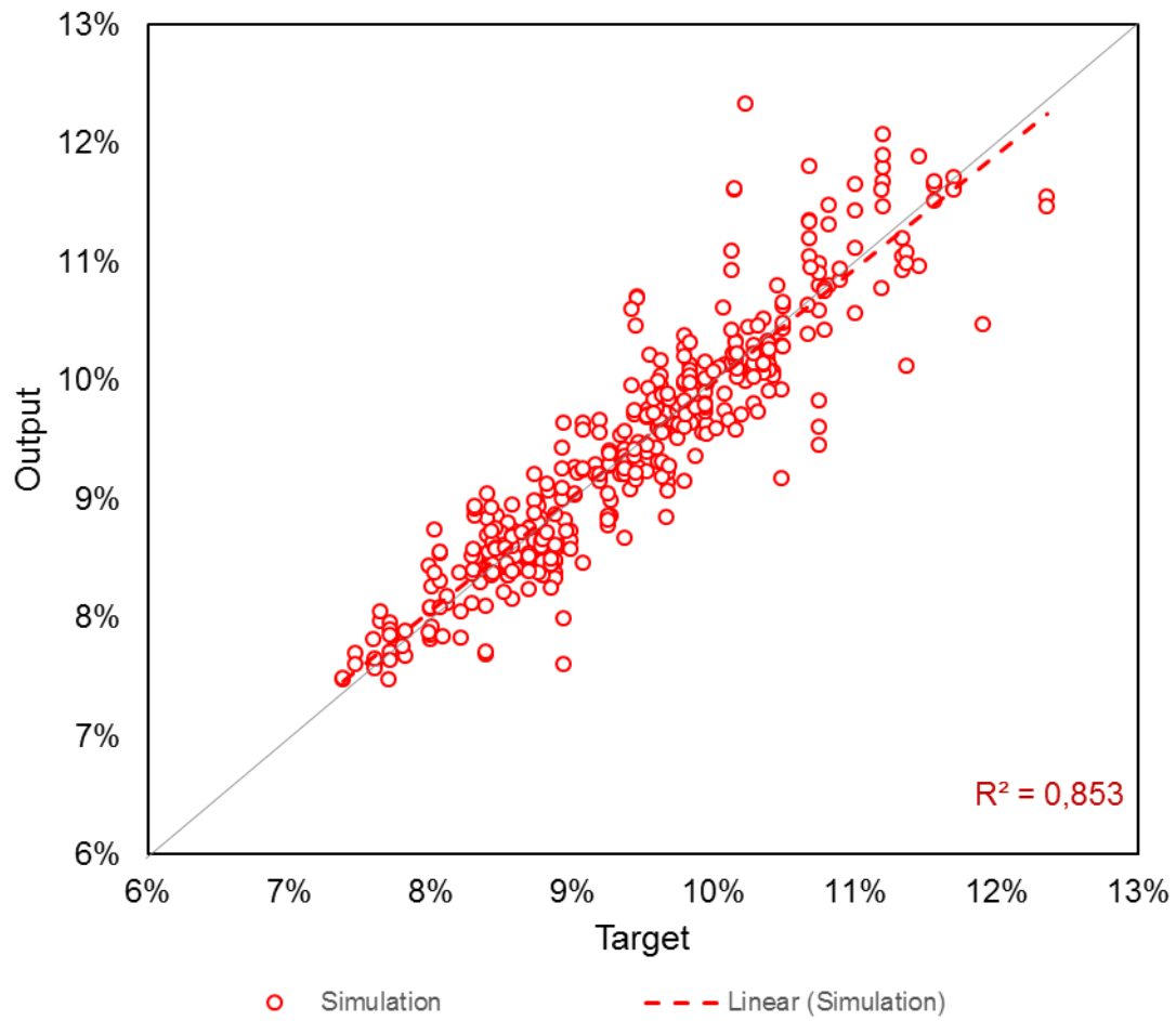
Figure E.2-2: Regression plot of the simulation of a 50-neuron neural network trained with the Bayesian regularisation algorithm using phase 2 porosity data
