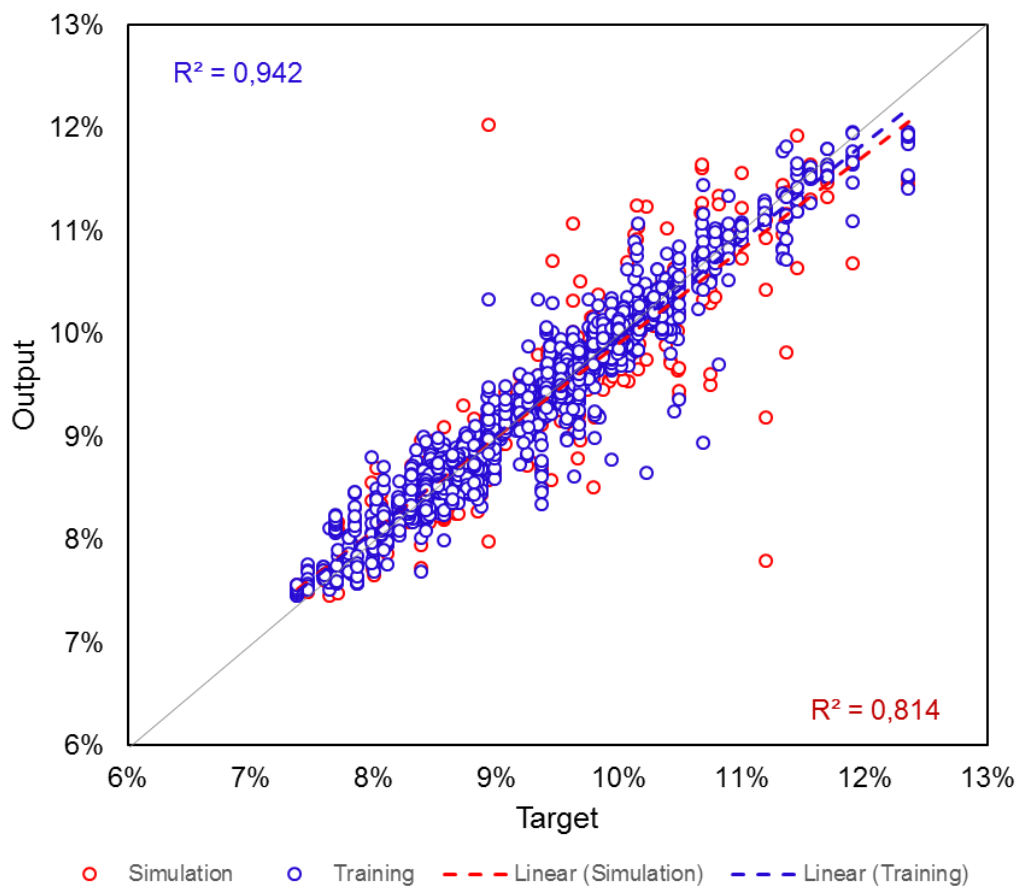
Figure 5.2-33: Regression plots of the training and simulation of a 61-neuron neural network trained with the Bayesian regularisation algorithm using phase 2 porosity data
