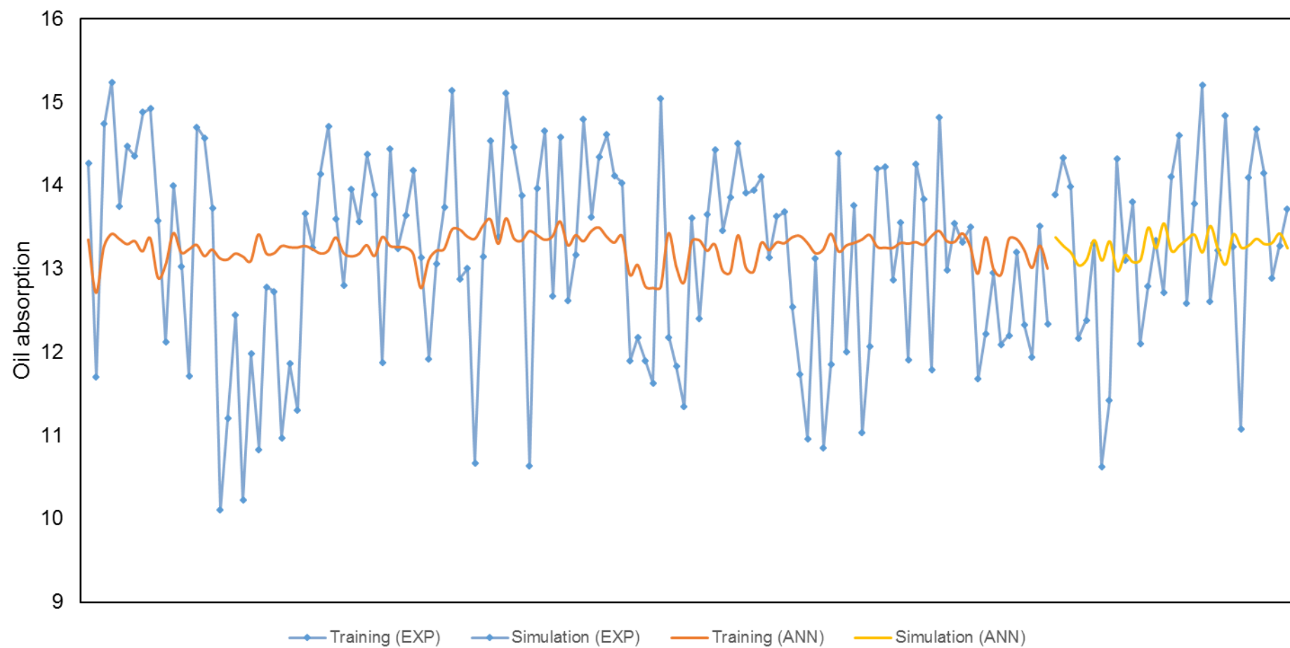
Figure 5.2-16: Model performance of a 100-neuron neural network trained with the Bayesian regularisation algorithm using discrete data
