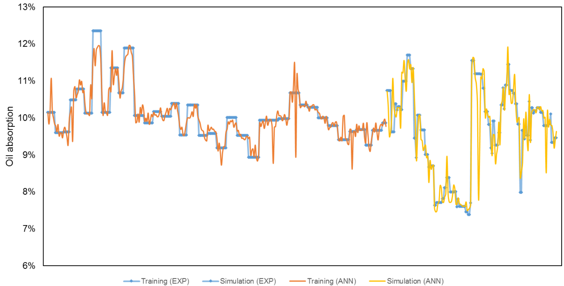
Figure 5.2-34: Model performance of a 61-neuron neural network trained with the Bayesian regularisation algorithm using phase 2 porosity data
