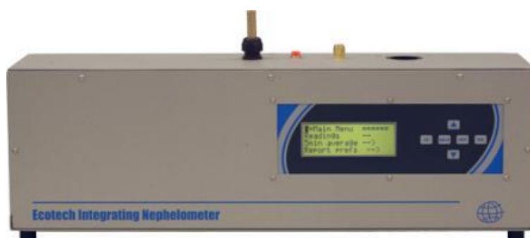
Figure 3-5: 3-wavelength nephelometer (Ecotech Aurora 3000) instrument
