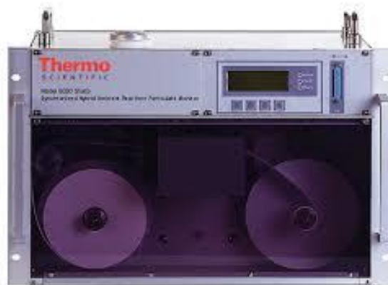
Figure 3-7: Synchronised hybrid ambient real-time particulate (SHARP) monitor (model 5030, Thermo Fisher Scientific Inc.) instrument
