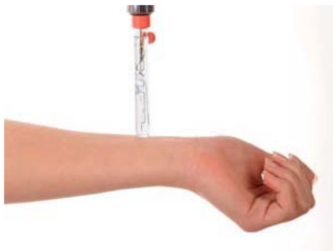
Figure E.5: Measurement with Skin-pH-Meter ® PH 905
