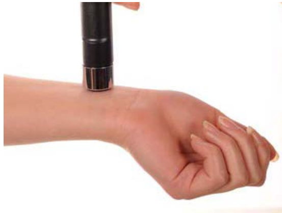
Figure E.4: Measurement with Mexameter ® MX 18
