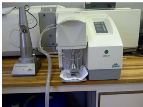
Figure D.4: Malvern Mastersizer 2000 with wet cell Hydro 2000 SM
