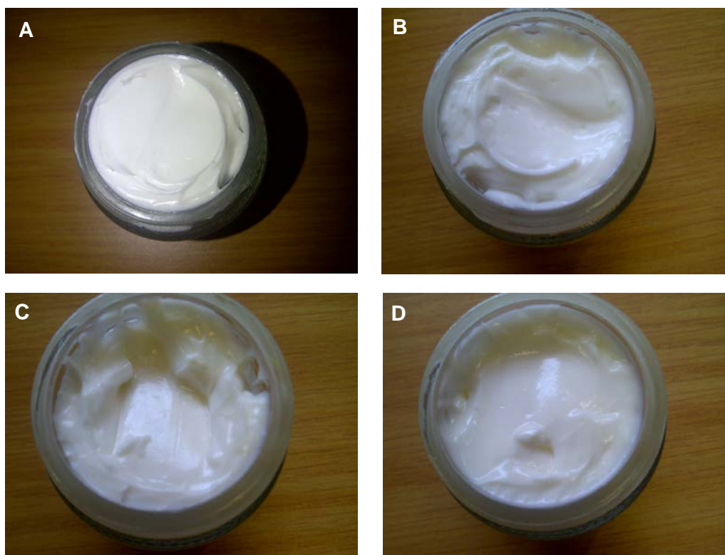
Figure D.10: The change in colour of cream stored in glass container from A) month 0 to month 6 at B) 25 °C/60% RH, C) 30 °C/60% RH and D) 40 °C/75% RH
