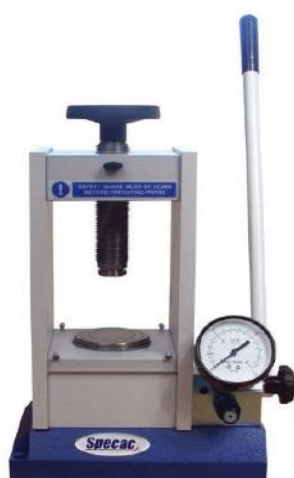
Figure 3-3: Specac's Atlas Series Manual Hydraulic Press
