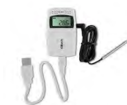
Figure 2-10: A Dual sensor data logger
