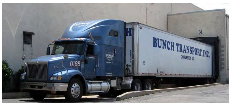
Figure 2-3: A refrigerated container (Reefer) connected to a temperature controlled loading dock
