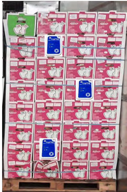
Figure 3-9: Sensors positions outside on boxes
