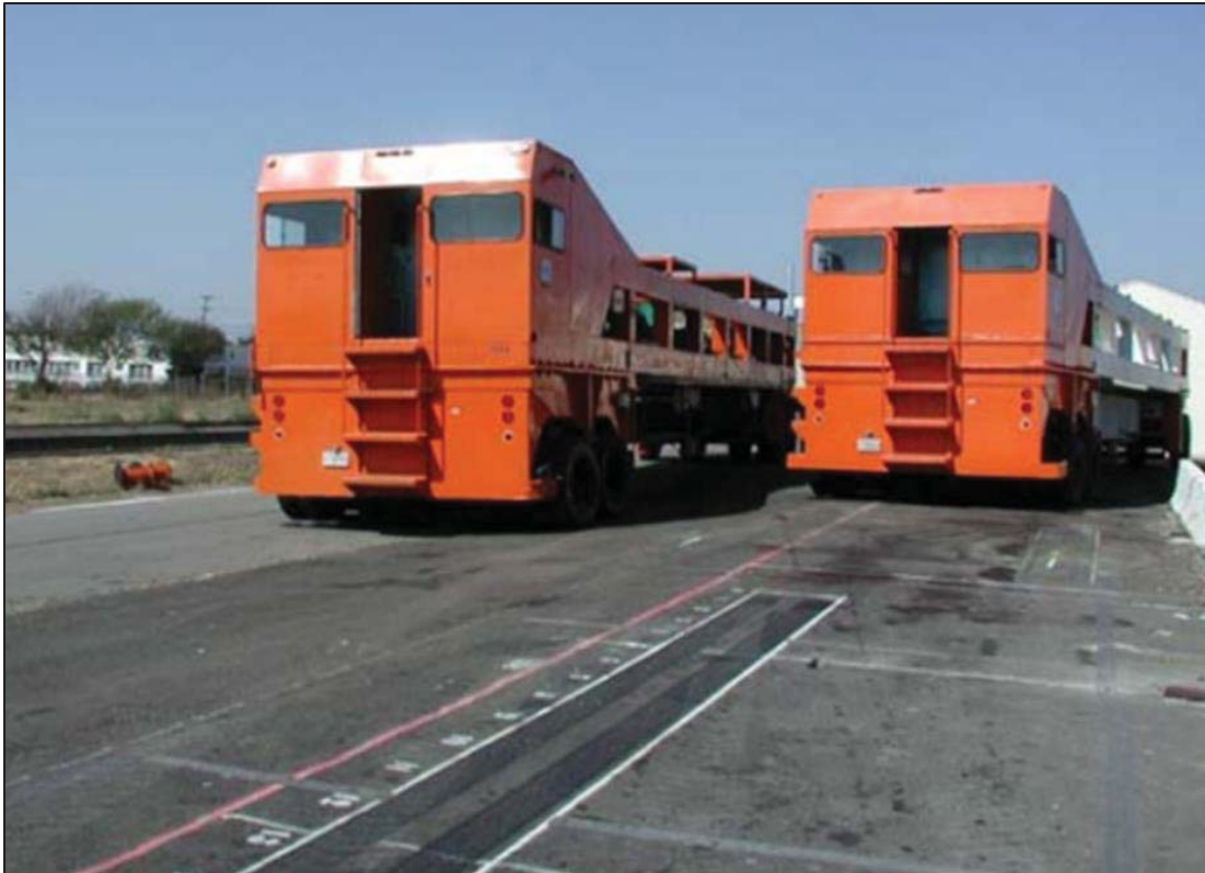
The two HVS units used in Berkeley, California for the evaluation of the I-710 innovative pavement designs
