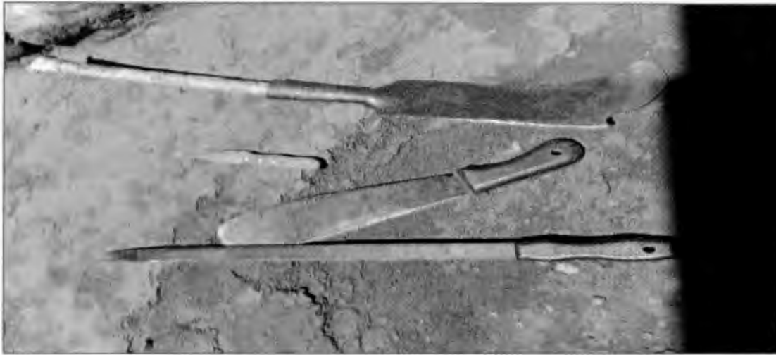
Figure 5.11: Tools used to harvest plants used for natural based cosmetics and cosmeceuticals (Non-ferrous metals including stainless steel Sharpener, Carbon Steel Hoe, and Machete)
