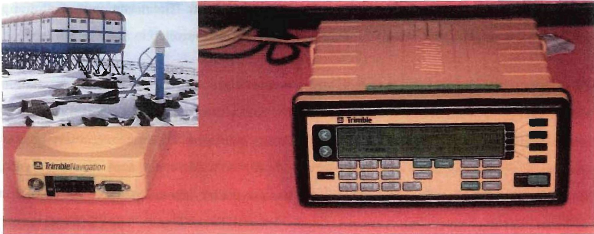
Figure 4.2: A photo of the GPS receiver at the SANAE IV base. The insert shows the antenna outside the base.
