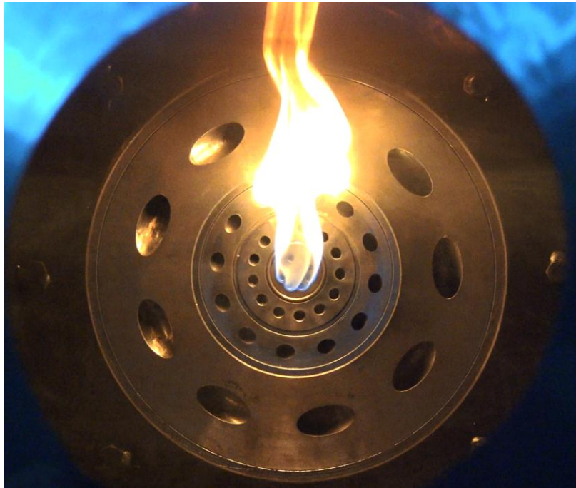
FIGURE 6.13: GAS FLAME WITH NO AIR SUPPORT
