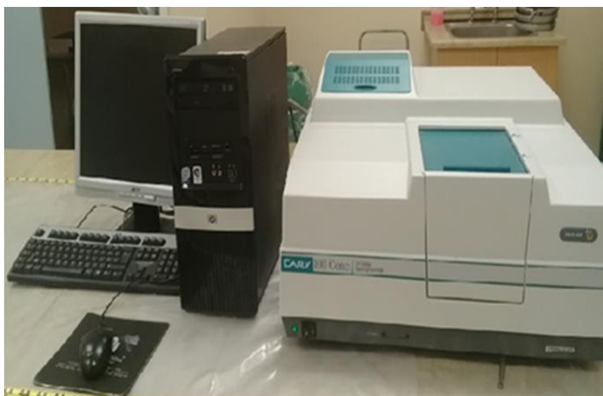
Figure 11: Ultraviolet Visible (UV Vis) Spectrophotometer used for uranium sample analysis at CARST
