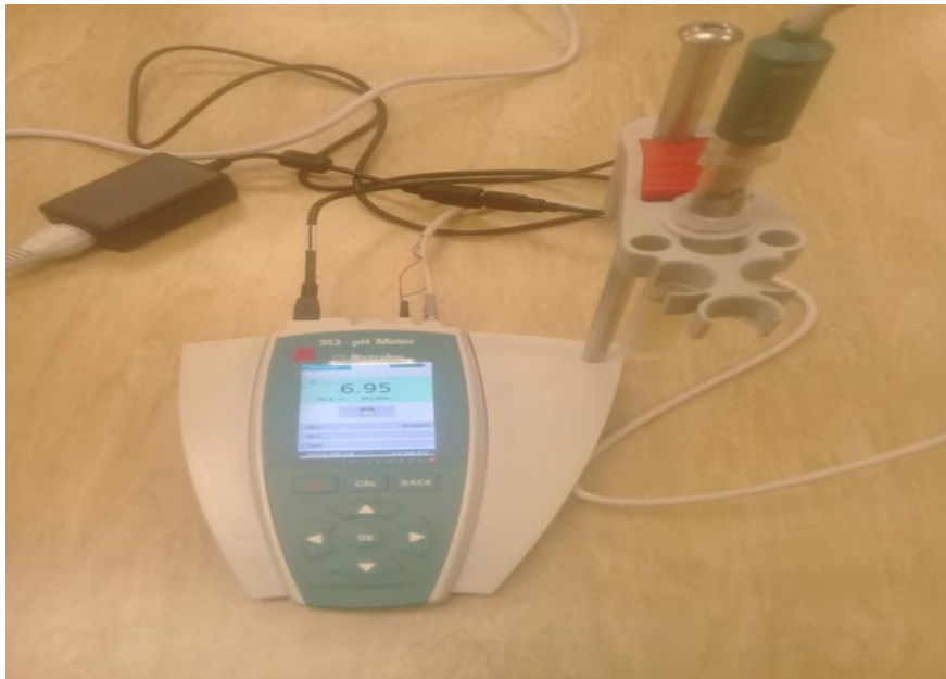
Figure 8: pH meter used for evaluation of pH in the carbonate solution
