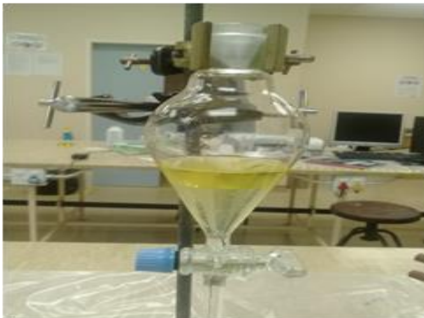
Figure 10: Experimental setup after solvent extraction (Uranium in Aliquat 336 and diluents)
