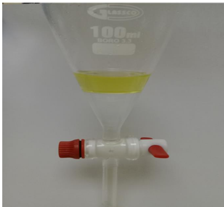
Figure 19: A 0.2 M of ammonium carbonate solution showing a colorless aqueous phase and yellow organic phase after extraction process
