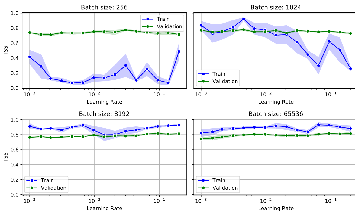
Figure 5.3: TSS versus LR plot for different batch sizes. No regularisation. 2_500 MLP architecture. Training set (blue), validation set (green).
