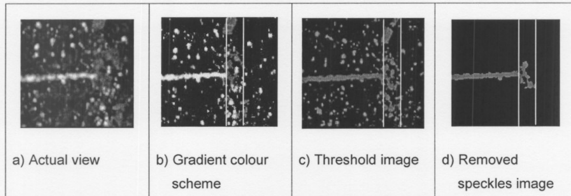
Figure 4-4: Cause of a faulty measurement.
