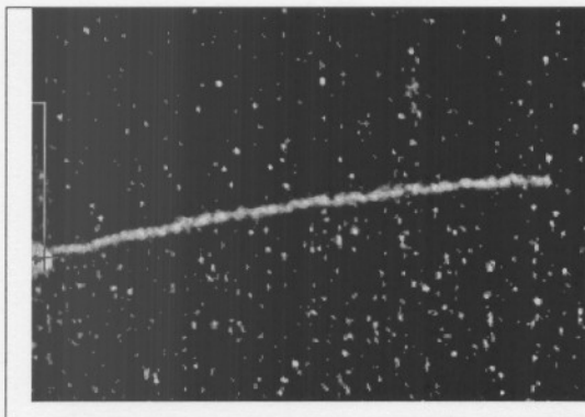
Figure 3-23: Crack length for mild steel.
