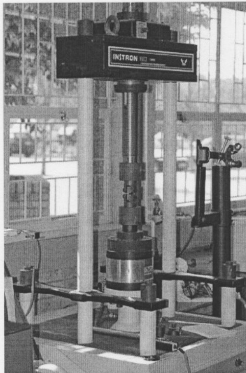
Figure 3-3: The Instron 1603 Electromagnetic Resonance (EMR) machine.
