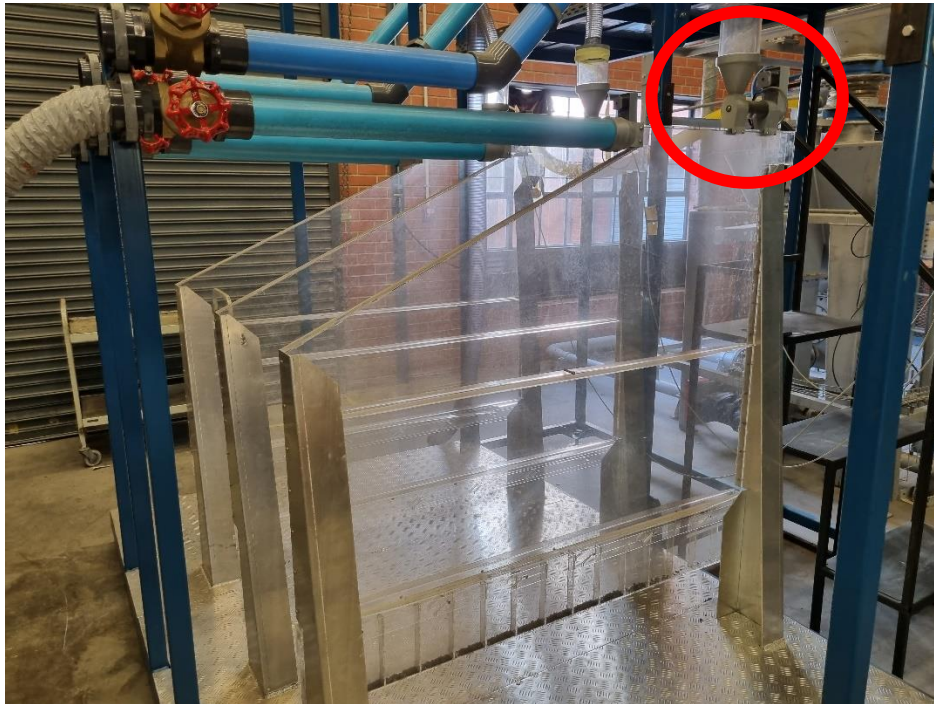
Figure 5.16 Density separation chamber close-up
