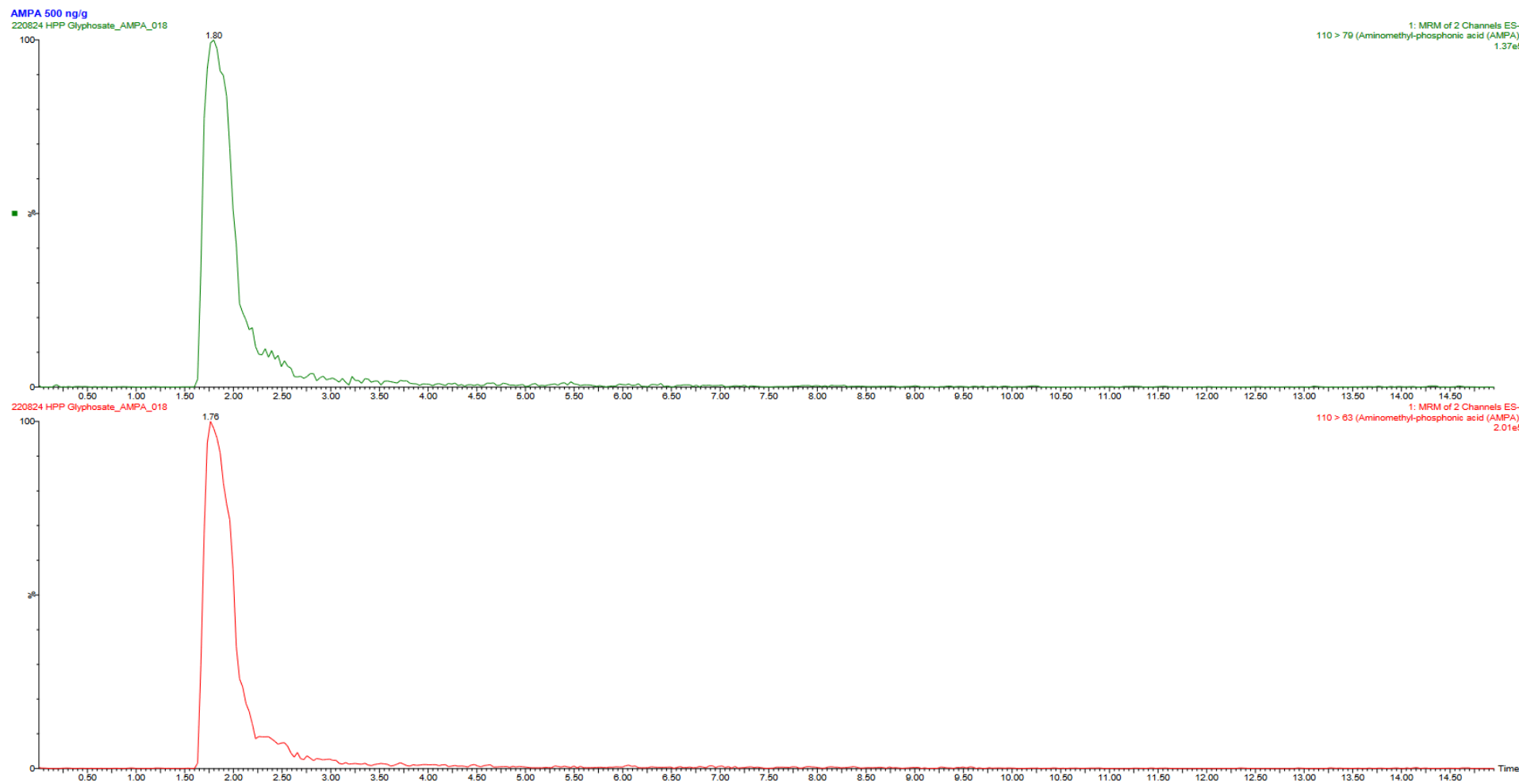
Figure 4.15: Multiple reaction monitoring (MRM) chromatogram for AMPA (aminomethylphosphonic acid) in extracted spiked water. Optimal recovery and adequate peak were observed. The two runs indicated by the repeatability of the peaks validate the analytical method.
