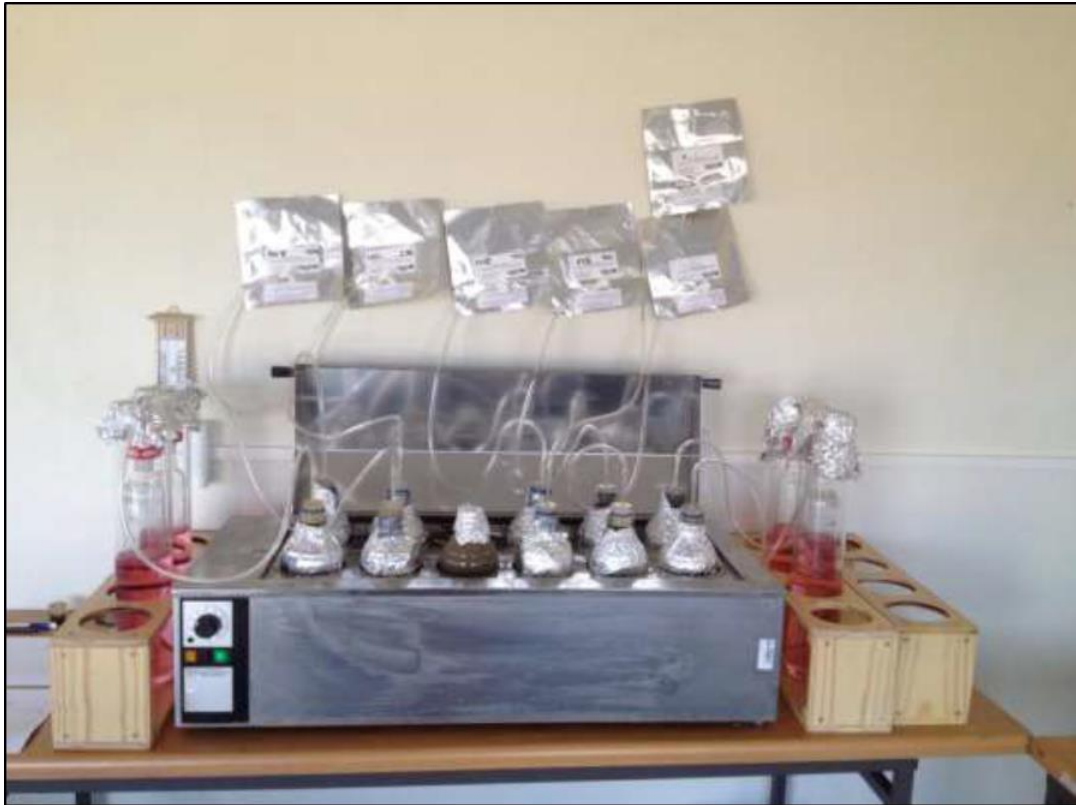
Figure 3-2: Experimental setup of bench top batch fermentation
