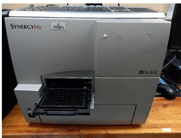
Figure 13. Synergy™ Mx Monochromator-Based Multi-Mode Microplate Reader
