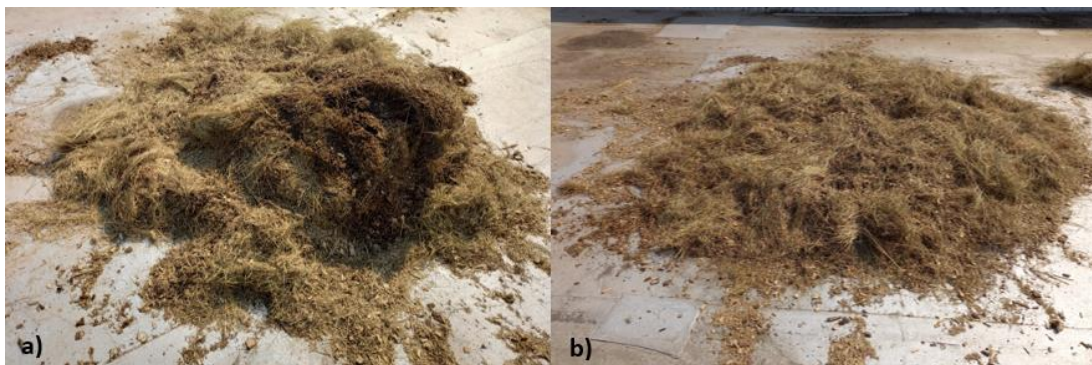
Figure 7. Photograph of bed material: a) before re-mixing; b) after re-mixing
