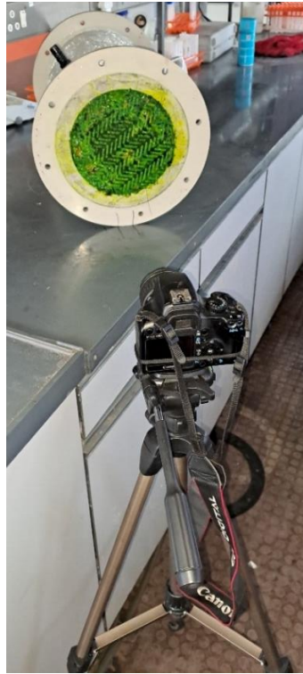
Figure 22. Camera setup for physical characterisation of the packed bed
