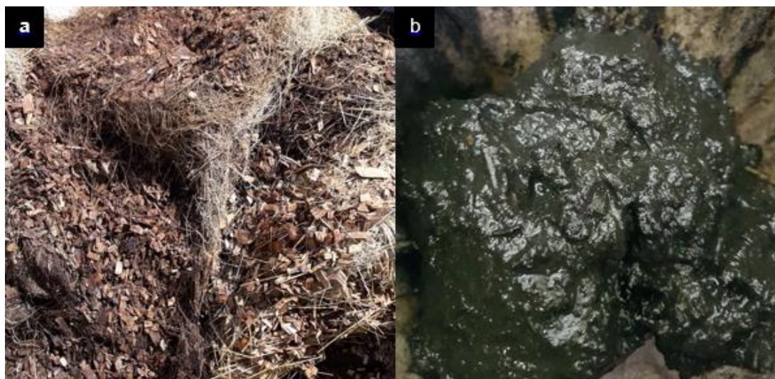
Figure 1. cloSURE® biological bed degradation, (a) before operation (large sample), (b) after 18 months of operation (500 mL sample)
