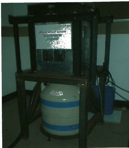
Figure 3.5: A photograph of high-purity germanium detector with accompanying lead castle at iThemba LABS Environmental Radioactivity Laboratory (ERL).
