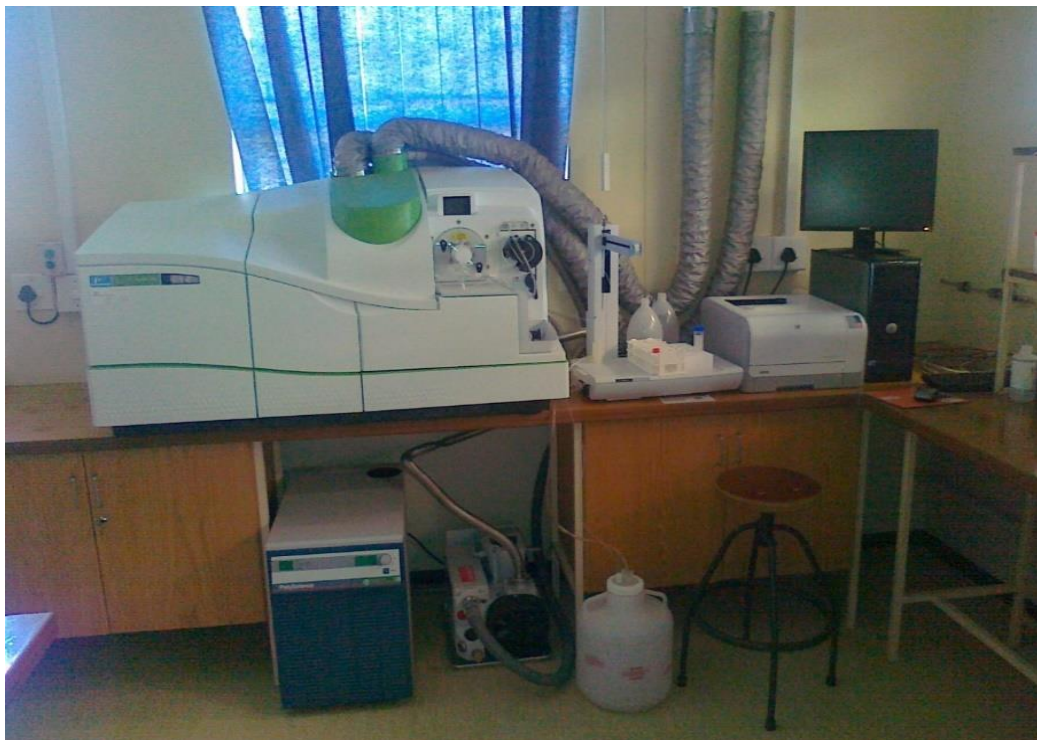
Figure 3.8: The NexION 2000C inductively coupled plasma - mass-spectrometry at CARST.
