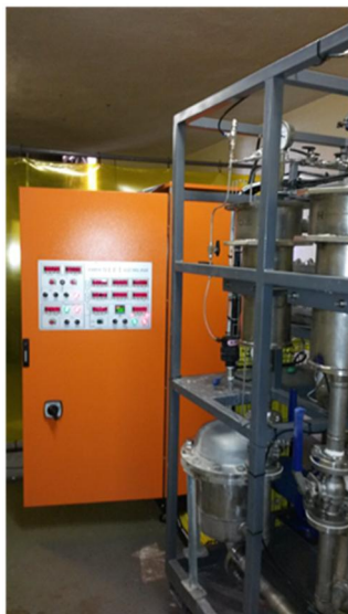
Figure 5-3: (a) HFP plant connected to the universal test panel, (b) HFP plant, and (c) assembled HFP reactor stack
