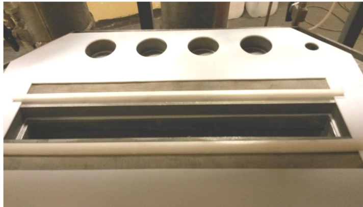
Figure 5-14: Uneven displacement of the rectangular electrodes due to the absence of a self-tensioning design
