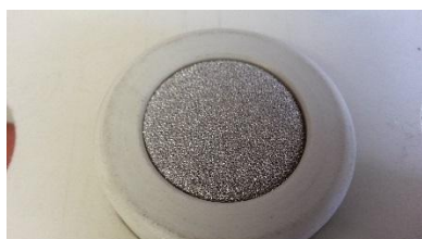
Figure 6-29: (a) nickel metal foam electrode, (b) a 80 µm nickel mesh electrode, and (c) a 200 µm nickel mesh electrode
