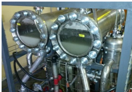
Figure 4-14: (a) Horizontal gas/liquid separator scale for the MCE plant in relation to the balance of plant, and (b) MCE plant gas/liquid separation system
