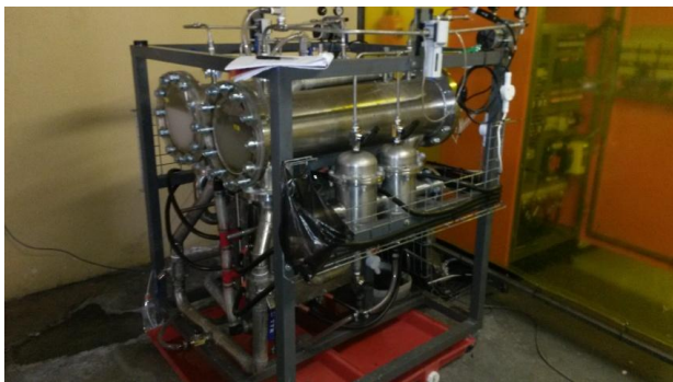
Figure 4-14: (a) Horizontal gas/liquid separator scale for the MCE plant in relation to the balance of plant, and (b) MCE plant gas/liquid separation system
