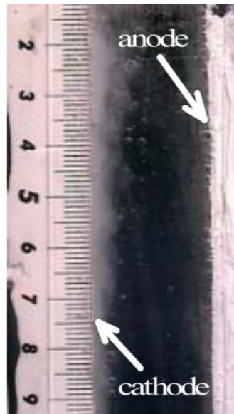
Figure 2-2: Expected bubble evolution profile from solid plate electrodes at a temperature of 40°C, 40% KOH, and 1 A.cm -2 [26]
