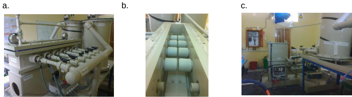
Figure 3-1: (a) DEFT™ concept optimisation test rig, (b) internals of the DEFT™ concept optimisation reactor, and (c) balance of DEFT™ concept optimisation test rig [6]
