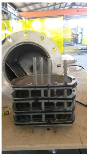
Figure 7-7: (a) Internals of a typical gas/liquid separation system used for the DEFT™ process illustrating the use of purge tubes, and (b) a translucent illustration of the effectiveness of removing micro-bubbles from a bi-phase solution by means of backed media and micronic filters
