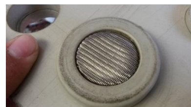
Figure 6-29: (a) nickel metal foam electrode, (b) a 80 µm nickel mesh electrode, and (c) a 200 µm nickel mesh electrode
