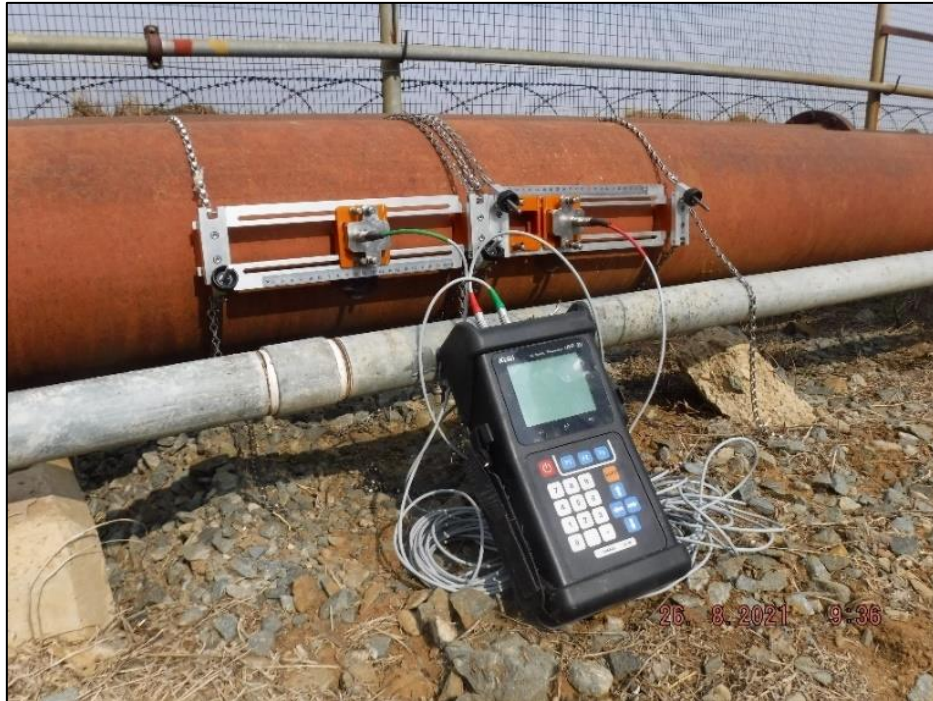
Figure 6: Clamp-on ultrasonic flow sensor 4
