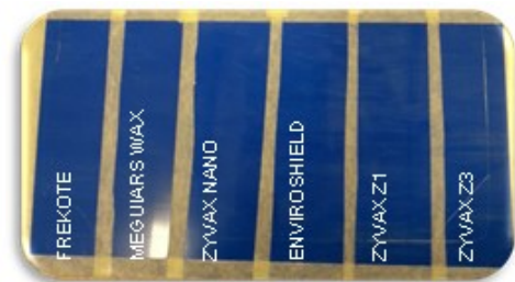
Figure 4-25: Test layout of the release agent test
