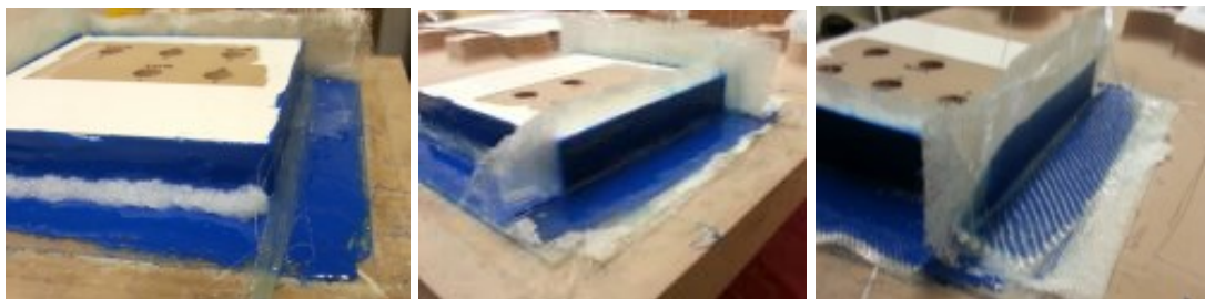
Figure 4-7: (a) Rovings and flox applied as strengthening methods; (b) Print barrier and glass 90070 applied with butt layup; (c) Glass 90070 applied as normal layup.
