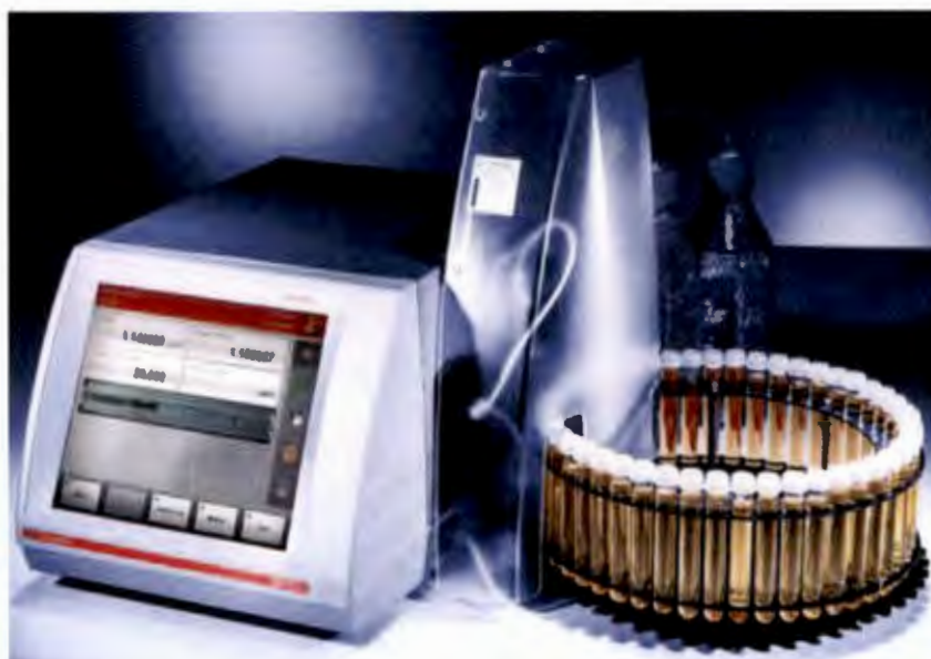
Fig 3.3 Photograph of Density and Sound Velocity Meter (DSA 5000 M) fitted with X-sample 452.
