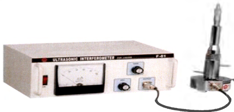
Fig 3.4 Photograph of the Mittal ultrasonic interferometer M-81G instrument. (Taken from the Instruction Manual of Mittal enterprises ultrasonic interferometer)
