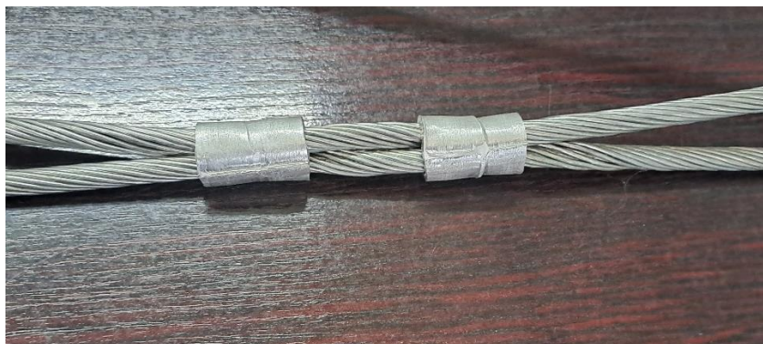
Figure 12: Ferrules used to connect two endpoints of wire ropes
