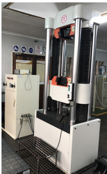
Figure 28: Sans universal tensile testing machine used in the tensile tests
