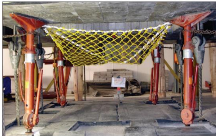
Figure 10: Polymer mesh after drop test (Skarbøvig et al. , 2011)
