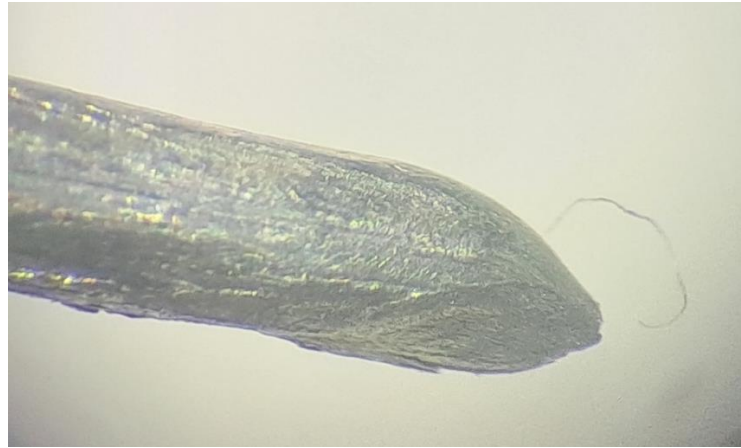
Figure 41: Wire rope ductile fracture
