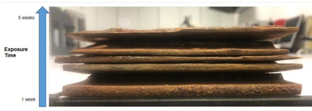
Figure 23: Thickness loss of carbon steel test specimens (Fortes et al. , 2022)
