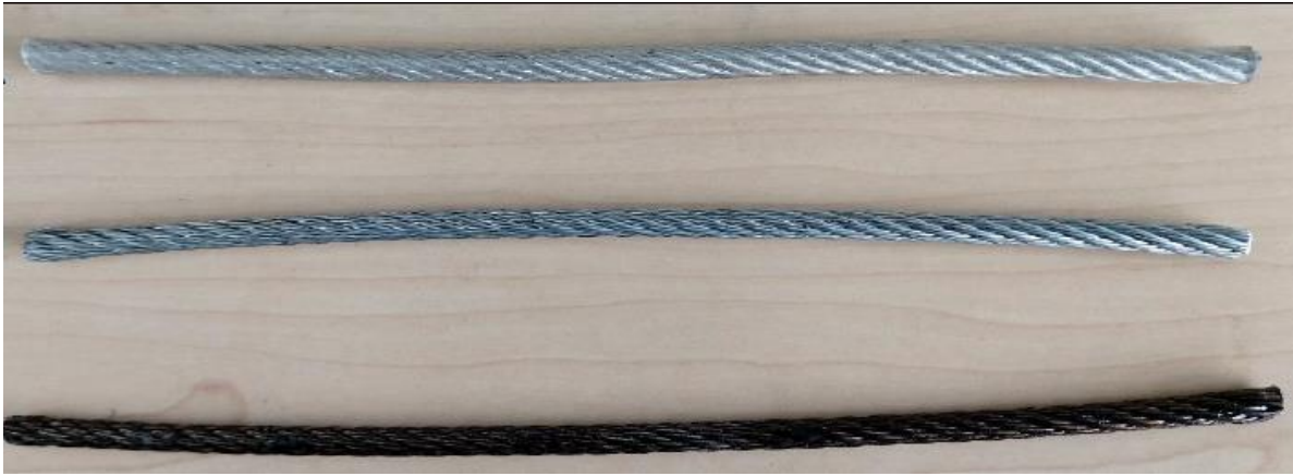
Figure 48: Galvanized PVC coated wire rope (top), galvanized wire rope (middle) and galvanized wire rope coated with bitumen (bottom) from MSP's wire mesh before salt spray test
