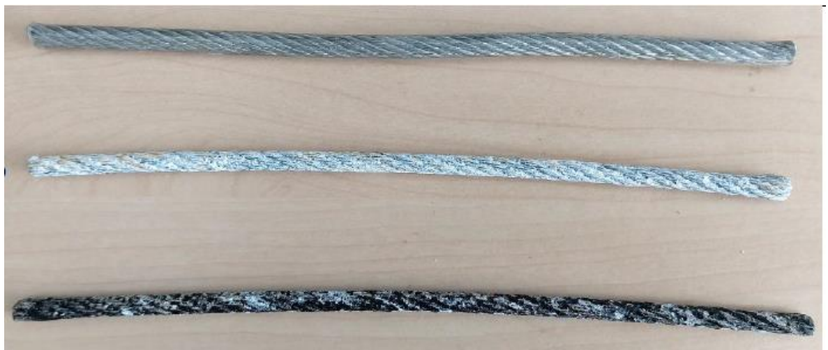
Figure 49: Galvanized PVC coated wire rope (top), galvanized wire rope (middle) and galvanized wire rope coated with bitumen (bottom) from MSP's wire mesh after salt spray test
