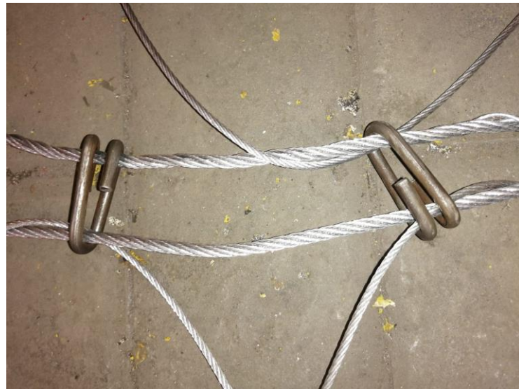
Figure 42: Rocnet connectors after drop test
