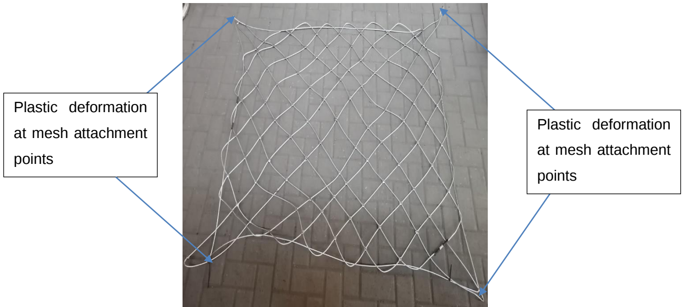
Figure 39: 4 mm (1x19) inner and outer wire rope mesh condition after a 300 mm drop test
