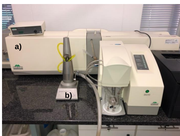
Figure B.10: a) Malvern Mastersizer 2000 Particle Size Analyser with b) a Hydro 2000SM Dispersion Unit
