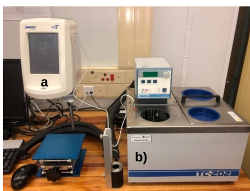
Figure B.14: a) Brookfield Viscometer DV2T LV Ultra, connected to b) a thermostatic water bath
