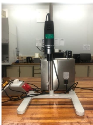
Figure B.1: High-energy emulsification method homogeniser (Heidolph Diax 600 Laboratory stirrer 240VAC)
