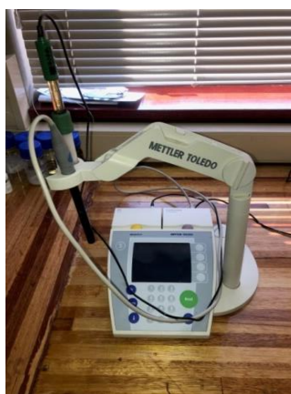
Figure B.5: A Mettler Toledo ® pH meter with a Mettler Toledo ® InLab ® 410 electrode
