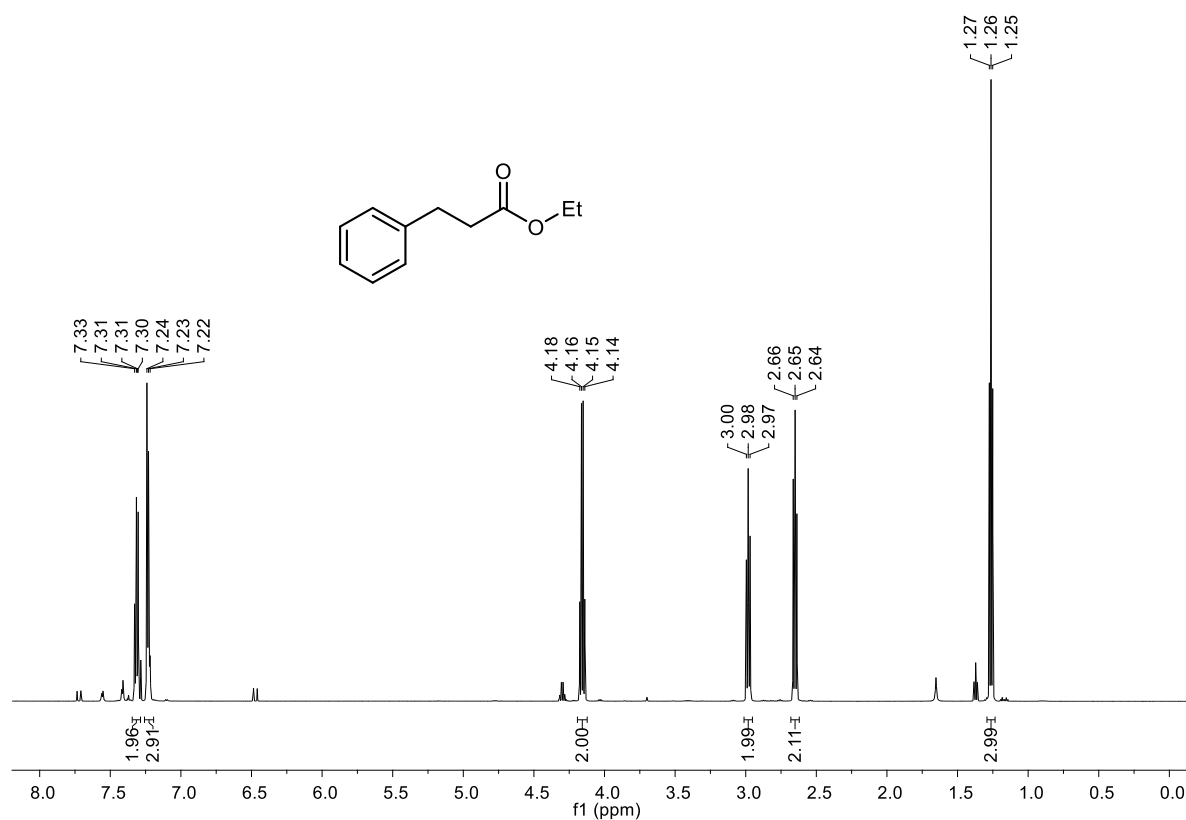
Figure S3.40 ^1\text{H} NMR (600 MHz, \text{CDCl}_3 ) spectrum of ethyl 3-phenylpropanoate.
