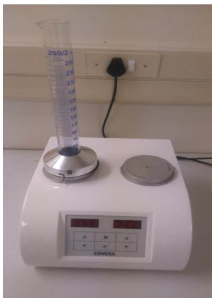
Figure 3.6: Image depicting the Erweka ® density apparatus
